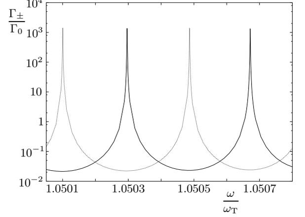
FIG. 3: The two-atom decay rates  $\Gamma_+ = \Gamma_{A'A'} + \Gamma_{A'A''}$  (solid curve) and  $\Gamma_- = \Gamma_{A'A'} - \Gamma_{A'A''}$  (dotted curve) for the symmetric and antisymmetric states, respectively, as functions of the transition frequency  $\omega$ , with  $\Gamma_{A'A''}$  from Eq. (114) for  $\theta = \pi$ . The other parameters are the same as in Fig. 2].
