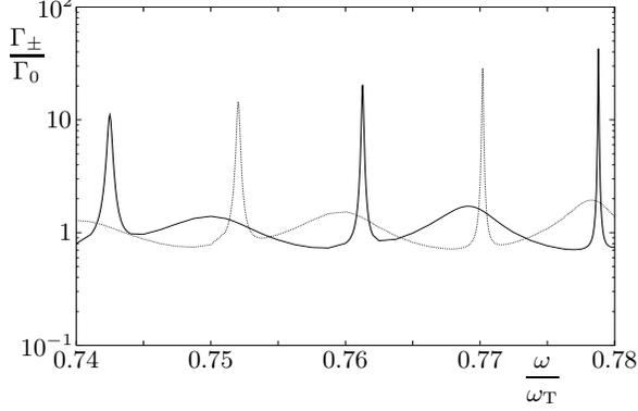
FIG. 5: The two-atom decay rates  $\Gamma_+ = \Gamma_{A'A'} + \Gamma_{A'A''}$  (solid curve) and  $\Gamma_- = \Gamma_{A'A'} - \Gamma_{A'A''}$  (dotted curve) for the symmetric and antisymmetric states, respectively, as functions of the transition frequency  $\omega$ , with  $\Gamma_{A'A''}$  from Eq. (114) for  $\theta = \pi$ . The other parameters are the same as in Fig. 2].
