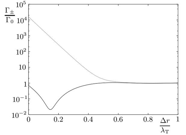
FIG. 4: The two-atom decay rates  $\Gamma_+ = \Gamma_{A'A'} + \Gamma_{A'A''}$  (solid curve) and  $\Gamma_- = \Gamma_{A'A'} - \Gamma_{A'A''}$  (dotted curve) for the symmetric and antisymmetric states, respectively, as functions of the distance  $\Delta r$  between the atom and the surface of the dielectric sphere, with  $\Gamma_{A'A''}$  from Eq. (114) for  $\theta = \pi$ . The other parameters are the same as in Fig. 2].
