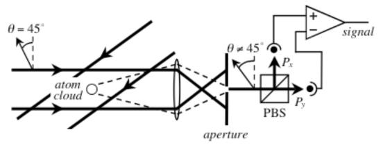
Figure 1. Setup for Faraday spectroscopy on atom samples in optical lattices. One of the linearly polarized lattice beams serves also as a probe beam, while an imaging lens and aperture ensures that only the part of the beam passing through the sample is detected. The polarization is analyzed by a simple polarimeter consisting of a polarization beamsplitter cube (PBS) and differential photo detector.
