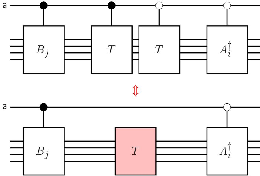
FIG. 11: Circuit for the measurement of spatial and time correlation functions. In this case  $\langle 2\sigma_+^a \rangle = \langle T^\dagger A_i T B_j \rangle$ . Notice the simplification achieved by reducing two C- $T$  operations into only one uncontrolled  $T$  operation.
