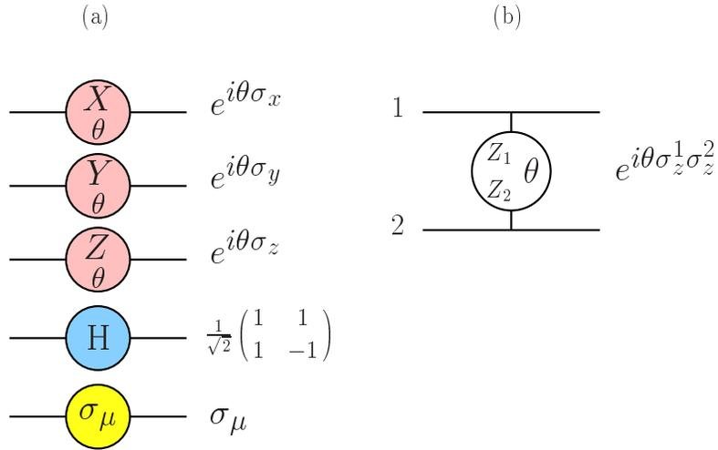
FIG. 3: (a) Some one qubit elementary gates and (b) a two qubit elementary gate.
