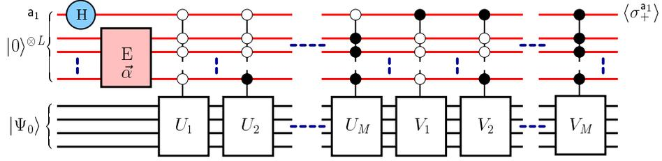
FIG. 10: Measurement of physical quantities using  $L$ -ancillas qubits  $\{a_1, \dots, a_L\}$ . In this case  $\langle \sigma_+^{a_1} \rangle = \frac{1}{2N} \langle \Psi_0 | [ \sum_{i=1}^M a_i U_i^\dagger V_i ] | \Psi_0 \rangle$  (see text).
