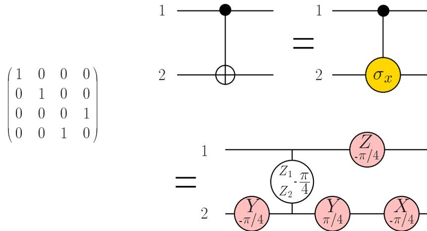
FIG. 5: C-NOT gate decomposition and its matrix representation. The control qubit is 1. Note that the last circuit realizes the C-NOT matrix operation up to a global phase  $e^{-i\frac{\pi}{4}}$ .
