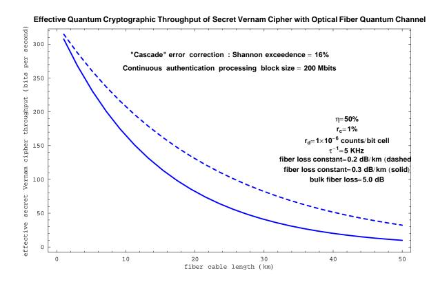
Figure 5: Effective throughput Rate Comparison for Single Photon Source with Fiber Cables of Two Different Qualities
