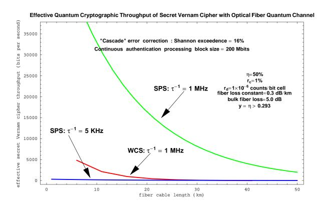
Figure 3: Effective Rate Curves for Fiber-Optic Link with Surreptitious Cable Replacement or use of Prior Shared Entanglement by Eve
