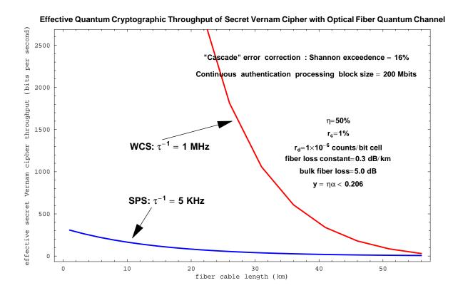
Figure 2: Effective Rate Curves for Fiber-Optic Link without Surreptitious Cable Replacement or use of Prior Shared Entanglement by Eve
