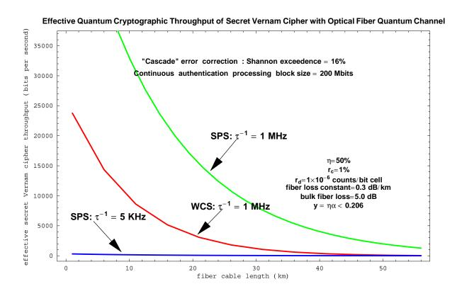
Figure 1: Effective Rate Curves for Fiber-Optic Link without Surreptitious Cable Replacement or use of Prior Shared Entanglement by Eve
