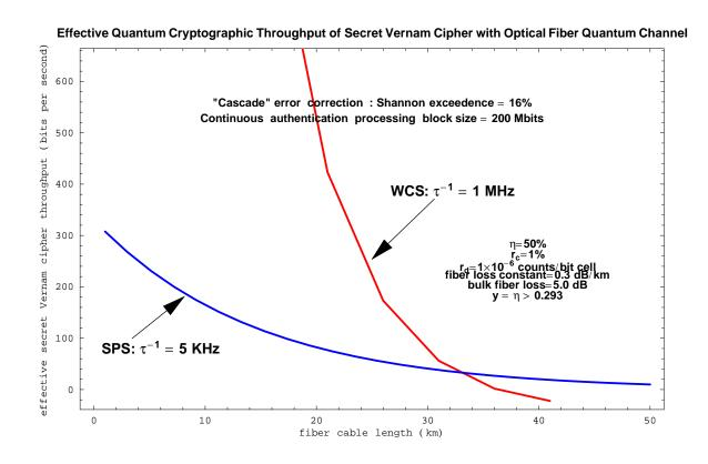
Figure 4: Effective Rate Curves for Fiber-Optic Link with Surreptitious Cable Replacement or use of Prior Shared Entanglement by Eve
