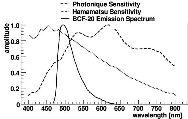
Fig. 1. Emission spectrum of a BCF-20 fiber [6] in comparison to the wavelength dependant response functions of a Hamamatsu SiPM (model MPPC S10361-025U) and a Photonic SiPM (model SSPM-0606EXP) [8]
