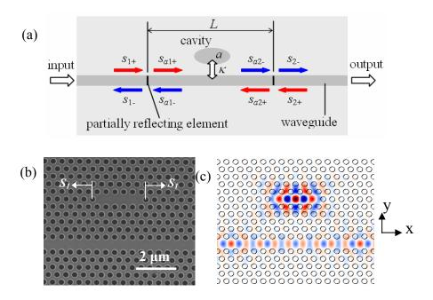
Fig. 1. (a) Schematic of optical system including a waveguide side-coupled to a cavity. Two partially reflecting elements are placed in the waveguide. (b) SEM of photonic crystal L5 point-defect cavity side-coupled to line-defect waveguide. The input and output facets of the high-index-contrast waveguide form the partially reflecting elements. (c)  $E_y$ -field of the resonance mode mid-slab from 3D FDTD simulations.
