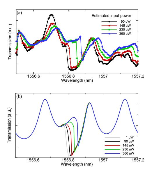
Fig. 2. Measured (a) and CMT-calculated (b) transmission spectrum at different input powers, illustrating the asymmetric lineshapes. The side-coupled L5 cavity has a total Q of  $\sim 30,000$ .
