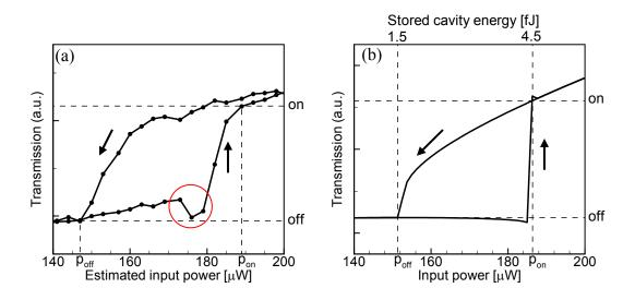
Fig. 3. (a) Measured and (b) CMT-calculated asymmetric hysteresis loops for Fano resonance at a detuning of 22 pm. The red-circled region in panel (a) highlights a dip in transmission with increasing input power, a signature not present in Lorentzian-type resonances, and indicative of nonlinear Fano-type solutions. The arrows depict ascending and descending input powers to the Fano system.
