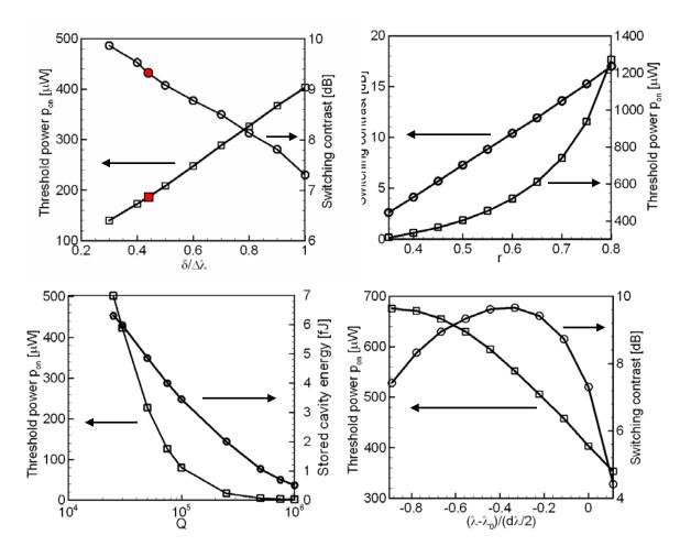
Fig. 4. CMT calculated effects of (a) the wavelength detuning  $\delta$ , (b) mirror reflectivity r, (c) cavity Q factor, and (d) the position of cavity resonance on the switching threshold power  $p_{on}$  and switching contrast. (The red-filled symbols correspond to the experimental parameters.)
