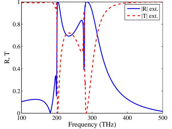
Fig. 5. Reflection and transmission coefficients calculated when the double array is represented as a slab of homogeneous material characterized by  $\epsilon_{\text{eff}}$ ,  $\mu_{\text{eff}}$  depicted in Fig. 4.
