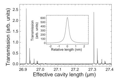
FIG. 3: Transmission of a 2FFP cavity versus cavity length. A piezo is used to vary the cavity length. The absolute length is determined by using up to three lasers as described in the text. The mirrors have radius  $1,000 \mu m$  with a stopband centered at 780 nm. The cavity has an effective cavity length of  $27 \mu m$  with a finesse of 1050; equivalently, free spectral range 5500 GHz and mode width (FWHM) 5.29 GHz. The inset shows the line shape of the fundamental (0,0) mode.
