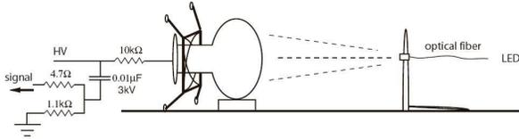
Figure 2. Schematic of the PMT test setup.
