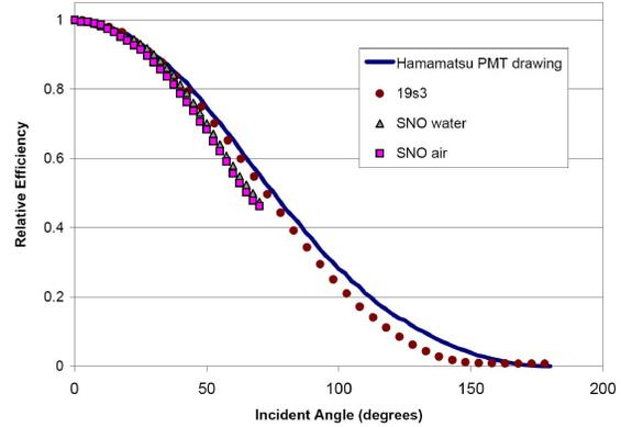
Figure 7. Response versus incident angle relative to the maximum at zero incidence angle. The prediction based solely on the PMT geometrical shape is compared with the MiniBooNE measurement in oil (tube 19s3 shown) and measurements in air and water from SNO.
