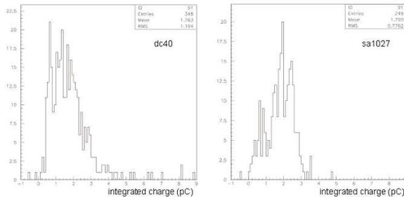
Figure 5. Integrated charge distributions for single photoelectron response for one R1408 (dc40) and one R5912 (sa1027) PMTs .
