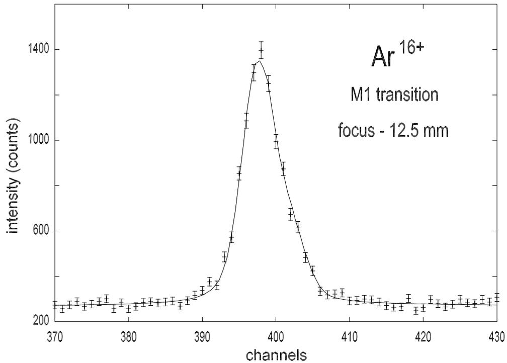
Fig. 3. The spectrum of the Ar<sup>16+</sup> 3104 eV M1 line measured with a quartz (10 $\bar{1}$ ) crystal is shown together with a fit for a detector position of 12.5 mm out of focus in direction of the crystal. A circular aperture with a diameter of 60 mm had been applied. One channel (pixel) corresponds to 93 meV.
