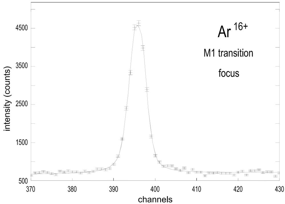
Fig. 4. The spectrum of the  $\text{Ar}^{16+}$  3104 eV M1 line measured with a quartz ( $10\bar{1}$ ) crystal is shown for the focal position together with a fit. A circular aperture with a diameter of 60 mm had been applied. One channel (pixel) corresponds to 93 meV.
