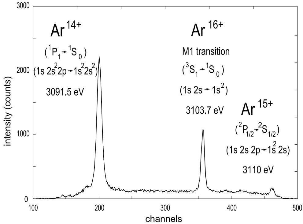
Fig. 2. The spectral region for argon X-rays from Ar<sup>14+</sup>, Ar<sup>15+</sup> and Ar<sup>16+</sup> (M1 transition) as emitted from the PSI ECRIT and measured with a Si (111) crystal. The energy values are from [7]. One channel (pixel) corresponds to 79 meV.
