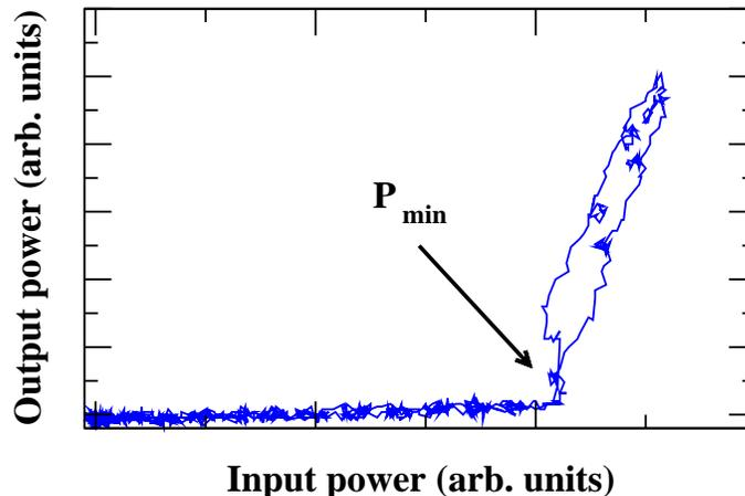
FIG. 5: Transfer function of the first cavity
