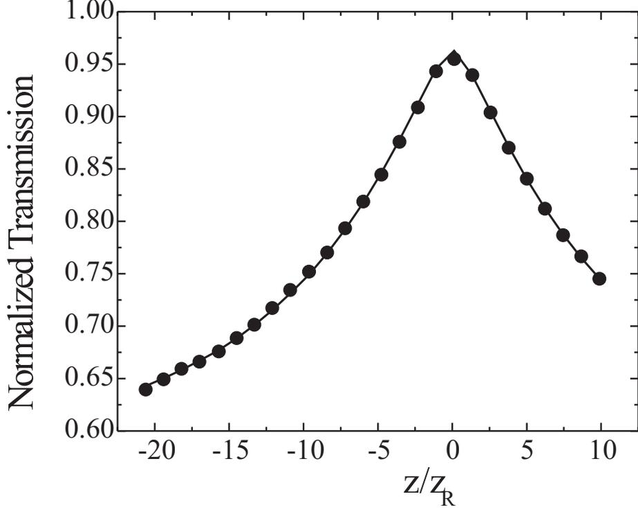
FIG. 2: Open-aperture scan at 300 MHz to the blue of the  $^{85}\text{Rb}$   $F=3 \rightarrow F'$  line, with fit from the Doppler-broadened two-level model. The scan at 300MHz to the red is very similar.
