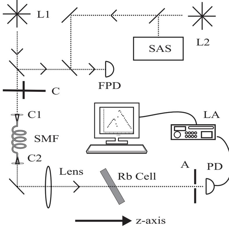
FIG. 1: Experimental configuration for the z-scan measurement. L1 and L2 = lasers 1 and 2; SAS = saturated absorption spectroscopy lock; C = chopper wheel; C1 and C2 = fiber coupling lenses; SMF = single mode fiber; A = aperture; PD = photodiode; LA = lock-in amplifier; FPD = fast photodiode.
