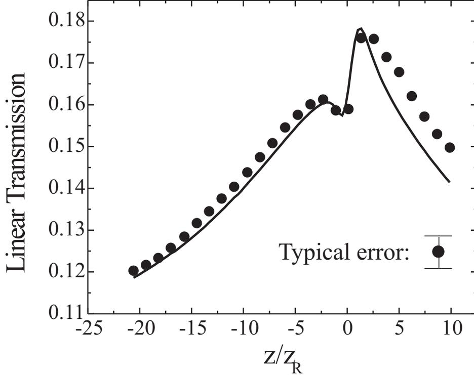
FIG. 3: Closed-aperture scan at 300 MHz to the blue of the  $^{85}\text{Rb}$   $F=3 \rightarrow F'$  line. The theory curve is calculated directly from the fit parameters found in the corresponding open scan, with no adjustable parameters. The typical systematic error mostly results from residual beam astigmatism and uncertainties about the aperture size.
