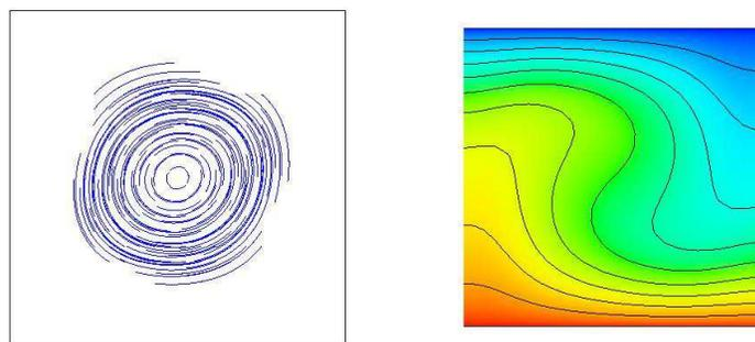
**Fig. 10:** Streamlines and temperature distribution for the bottom-heated buoyant cavity flow at  $Ra = 10^4$ .
