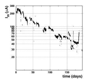
Figure 6. Current for RPC A corrected for temperature (see text) plotted versus time. The detector was placed at about 55 cm from the source.
