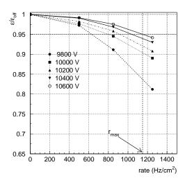
Figure 7. Efficiency vs. rate for RPC A, at different  $V_0$  values, measured in August 2001. The rate capability  $r_{max}$  is defined in the text.
