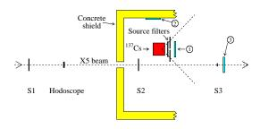
Figure 1. Schematic view of the test setup (not to scale). The positions of the RPCs corresponding to the various measurements are indicated (1-3). The distance of the RPC from the source in position 1 was about 55 cm, and in position 3 about 140 cm. The scintillator counters (S1-S3 and the Hodoscope) were used for measuring the RPC efficiency with the particle beam.
