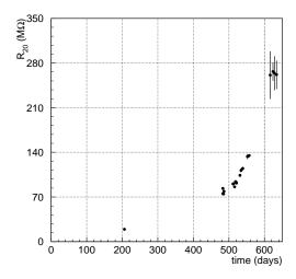
Figure 4. Measurements of R for RPC A versus time. The time scale starts at the beginning of the aging test in January 2001
