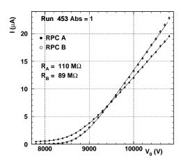
Figure 2. Current vs.  $V_0$  for RPC A (solid circles) and B (open circles) for absorption factor 1. The effective resistances  $R_{\rm eff}$  as obtained from the slopes are also shown. In this case we had  $X=49.8\pm8.9$ .
