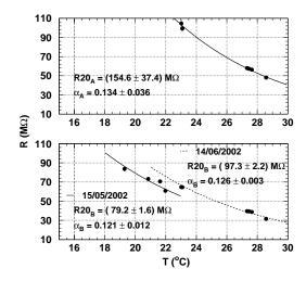
Figure 3. Resistances of RPC A and B plotted versus temperature. The temperature coefficient  $\alpha$  is fitted using an exponential dependence [18].
