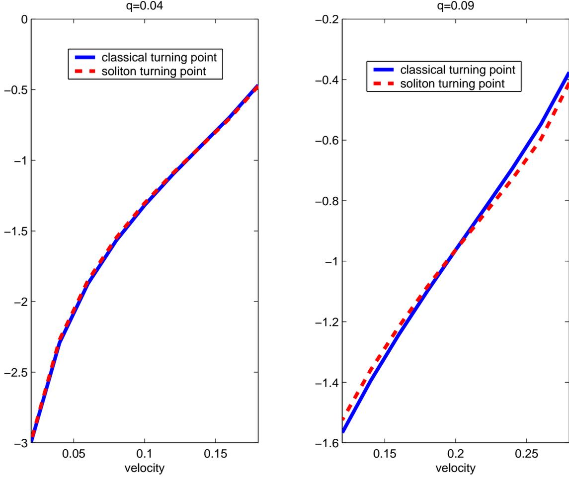
FIGURE 3. Two plots with  $q = 0.04$  and  $q = 0.09$ , respectively, and  $a_0 = -10$ . The blue line is the theoretical prediction of the turning point of the soliton,  $|a_{\text{turn}}| = \text{sech}^{-1}(v/\sqrt{q})$ , and the red dashed line is the actual soliton turning point. For smaller values of  $q$  the agreement is outstanding.
