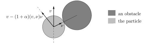
This mapping changes only the normal component of v, i.e.,  $(v, \nu)\nu$ , which is multiplied by  $-\alpha$ . On the figure, the dotted line indicates the trajectory of the particle's center.
