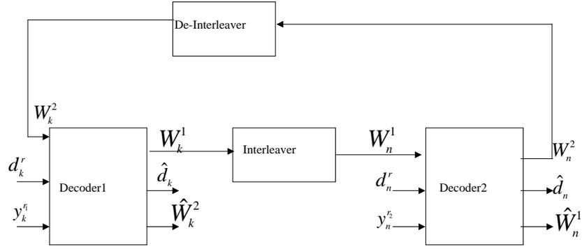
Figure 1: Structure of a Turbo decoder.
