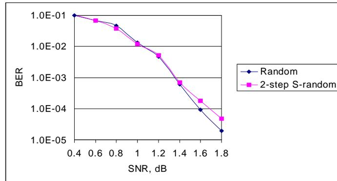
Figure 4: Performance of Turbo code for different interleavers of size 1024 bits and QPSK signal.
