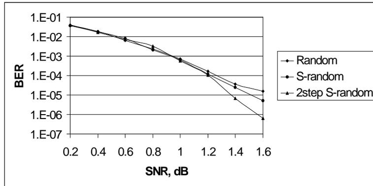
Figure 3: Performance of Turbo code for different interleavers of size 400 bits and BPSK signal.
