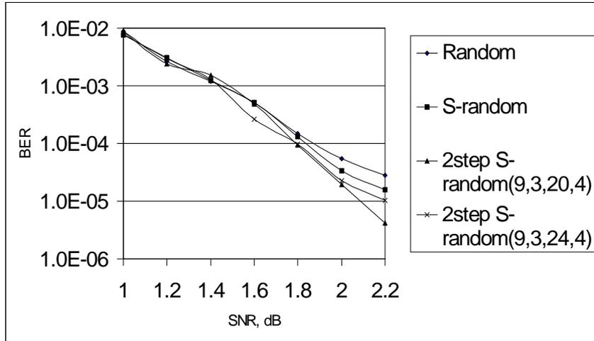
Figure 2: Performance of Turbo code for different interleavers of size 192 bits and BPSK signal.
