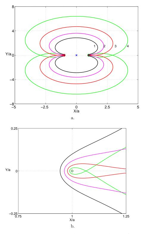
Figure 4: Equilibrium domains. Flow is driven by a quadrupole of moment  $\beta$  and two electric charges Q located at  $z=\pm a$ ; plots correspond to  $\beta=1$ ; Q=1; and  $A=0.2677;~0.3183=1/\pi;~0.3785;~0.4502$  for curves 1-4 respectively (a). Blowup of Fig.4,a. The charge remains outside the equilibrium domain; only non-intersecting boundaries correspond to physically admissible equilibrium domains.
