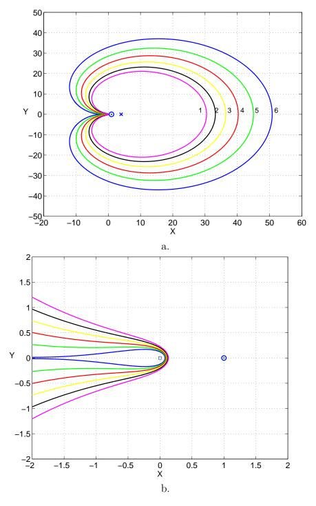
Figure 1: Equilibrium domains. Flow is driven by a source at z=a, and sink at z=b, an electric charge Q is located at z=0; plots correspond to q=1; a=1; b=4; and Q=0.2734, 0.2959, 0.3189, 0.3424, 0.3664, 0.3909. for curves 1-6 respectively (a). Figure (b) shows blow-up of the upper figure illustrating that the electric charge is outside the equilibrium domain.
