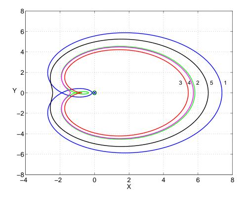
Figure 3: Equilibrium domains. Flow is driven by a dipole of moment  $\mu$  and an electric charge Q located at z=0; plots correspond to  $\mu=1$ ; Q=1; and  $A=1,\sqrt{2},2,2\sqrt{2},$  and 4 for curves 1-5 respectively. Self-intersecting boundaries 1 and 2 correspond to non-physical domains.
