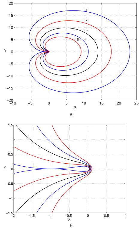
Figure 2: Equilibrium domains. Flow is driven by a dipole of moment  $\mu$  at z=a, an electric charge Q is located at z=0; plots correspond to  $\mu=1$ ; a=1; and Q=0.2026; 0.2410; 0.2866; 0.3408; 0.4053. for curves 1-5 respectively (a). Figure (b) shows blow-up of the upper figure illustrating that the electric charge is outside the equilibrium domain.
