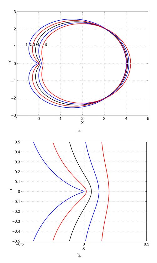
Figure 6: Equilibrium domains for flow driven by a dipole in quadratic axisymmetric external potential field for B=2.0;2.0212.061;2.121;2.201 (curves 1-5 respectively), (a); blow-up of Fig.6,a, (b).
