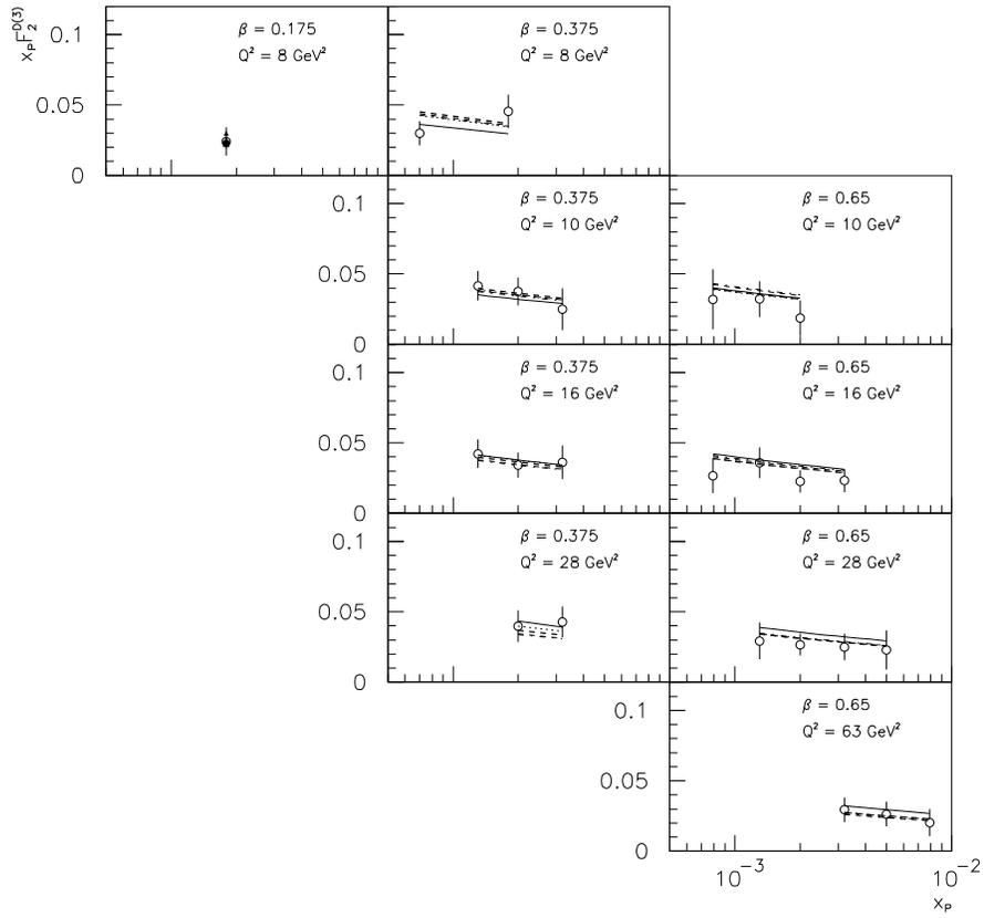
FIG. 2. Comparison of the fits for  $\alpha_{\mathbb{P}} = 1.14$  and the DIS data from ZEUS [6, 7] that were used in the fits. The LPS data we used consist of just the three points at  $Q^2 = 8 \text{ GeV}^2$ . The code for the lines is the same as in Fig. 1.
