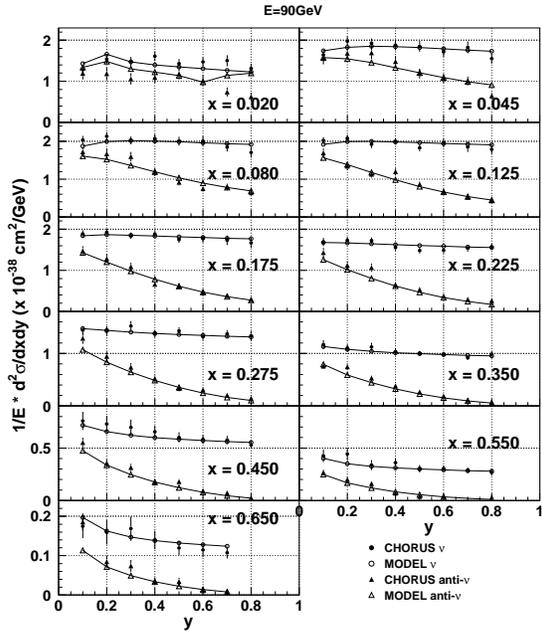
Figure 4. Comparison of our calculation (open symbols) with CHORUS data [11] (full symbols) for neutrino (circles) and antineutrino (triangles) differential cross-sections on  $^{207}\text{Pb}$  at  $E = 35\text{ GeV}$  (upper plot) and  $E = 90\text{ GeV}$  (lower plot).
