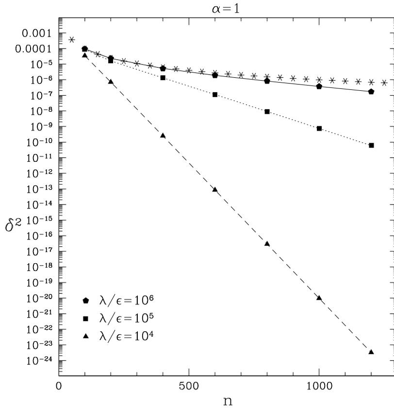
Figure 2: The (squared) deviation norm  $\delta^2$  of the polynomial approximations of  $x^{-1}$  as function of the order for different values of  $\lambda/\epsilon$ . The asterisks show the  $\epsilon/\lambda \rightarrow 0$  limit.
