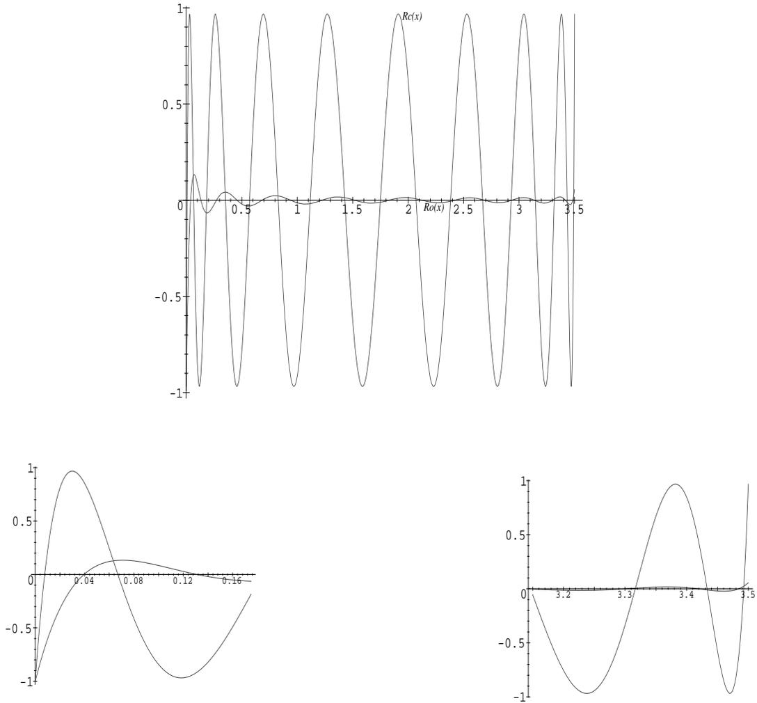
Figure 1: The comparison of the relative deviation  $R(x) \equiv xP(x) - 1$  for the Chebyshev polynomial ( $Rc(x)$ ) and the quadratically optimized polynomial ( $Ro(x)$ ). In the lower part the two ends of the interval are zoomed.
