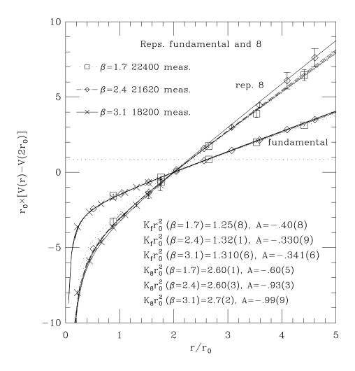
FIG. 2. The static quark potential V(R) in terms of hadronic scale  $r_0$  for representations fundamental and 8. The double line shows the central value of the fit  $\pm$  error. The horizontal dotted line shows the potential energy of glue-lumps. Good scaling behavior is observed. The weighted average string tensions for representations fundamental and 8 are  $Kr_0^2=1.324(4)(51)$  and  $Kr_0^2=2.602(9)(119)$ , respectively.
