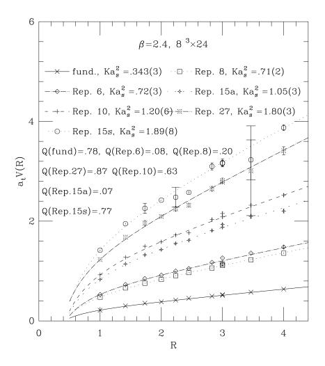
FIG. 4. A typical plot of  $a_t V(R)$  versus R for various representations  $8^3 \times 24$  lattice at  $\beta = 2.4$ .  $Ka_s^2$  shows the string tension times the spatial lattice spacing square. The error bars on the points are the sum in quadrature of statistical and systematic errors. The systematic errors are due to a change of the fit range of V versus T.
