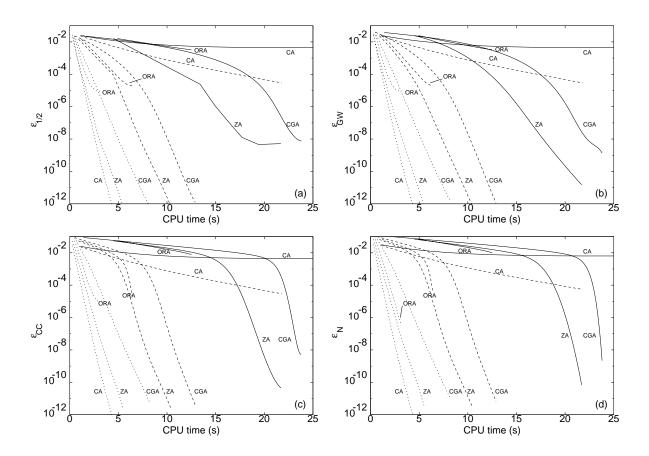
FIG. 4: Error limits as a function of the CPU time taken on a Fujitsu VPP5000— (a)  $\epsilon_{1/2}$ , (b)  $\epsilon_{GW}$ , (c)  $\epsilon_{CC}$  and (d)  $\epsilon_{N}$ . In each case the dotted line is for configuration A ( $\kappa = 10^{3}$ ), the dashed line for configuration B ( $\kappa = 4.4 \times 10^{5}$ ) and the full line for configuration C ( $\kappa = 3.6 \times 10^{9}$ ).
