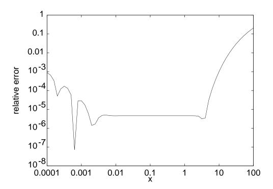
FIG. 2: The relative error,  $|\epsilon(z)|\sqrt{z}$ , in the ORA with  $N_O = 14$  fitted to the range [0.01, 1] for computation in and outside the range.
