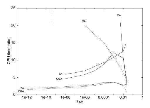
FIG. 7: The ratio of CPU time taken at fixed error,  $\epsilon_{1/2}$ , for (a) configurations B and A (dashed lines) and (b) configurations C and A (full lines) for three different algorithms.
