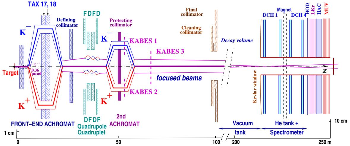
Figure 1: Schematic lateral view of the NA48/2 beam line (TAX17,18: motorized beam dump/collimators used to select the momentum of the  $K^+$  and  $K^-$  beams; FDFD/DFDF: focusing set of quadrupoles, KABES1–3: kaon beam spectrometer stations), decay volume and detector (DCH1–4: drift chambers, HOD: hodoscope, LKr: EM calorimeter, HAC: hadron calorimeter, MUV: muon veto). Note that the vertical scales are different in the two parts of the figure.
