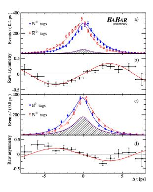
Figure 1. Measured decay-time distributions and corresponding decay-rate asymmetries for the  $BABAR \sin 2\beta$  analysis. a) and b) CP odd finals states, c) and d) CP even final state. The shaded regions represent the estimated background contribution. The solid (dashed) curves represent the fit projections in  $\Delta t$  for B ( $\overline{B}$ ) tags.
