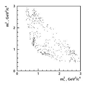
Figure 2. Dalitz plot distribution  $m_-^2=m_{K_S^0\pi^-}^2$  versus  $m_+^2=m_{K_S^0\pi^+}^2$  as measured in the Belle  $B^0/\overline{B}{}^0 \to D^0/\bar{D}{}^0h^0$  analysis.
