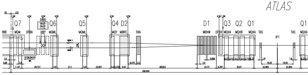
Figure 3: Schematic layout of the LHC LSS1 near the ATLAS interaction point showing the location for the RP units in the region between the Q6 and Q7 quadrupoles.
