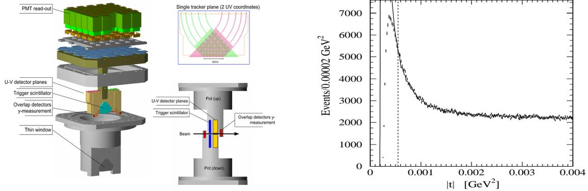
Figure 5: Left: Schematic view of the fiber tracker and the pot assembly. Right:  $dN/dt$  distribution of simulated reconstructed events as a function of the reconstructed  $-t$  value. A fiducial cut of  $\pm 45$  degree in azimuthal coordinate was applied. The solid line indicates the fitted region from  $0.00055 \leq |t| \leq 0.03 \text{ GeV}^2$ .
