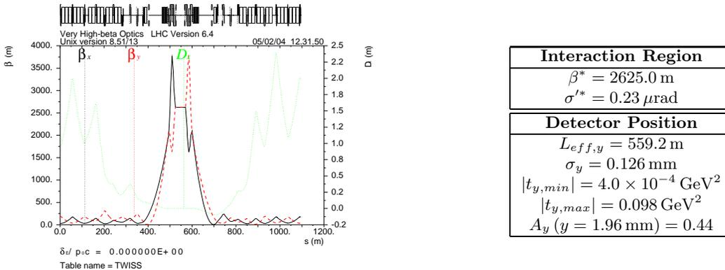
Figure 4: The optics diagram around IP1 for the very high-beta,  $\beta^* = 2625$  m, optics solution. The main beam parameters are also shown at the ATLAS IP and at the RP detector location at 240 m distance. The beam parameters were calculated using a normalized transverse emittance of  $1 \mu\text{m rad}$ .
