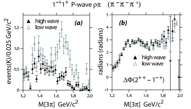
FIG. 25: (a) The  $1^{-+}1^{+}$  P-wave  $\rho\pi$  partial wave in the charged mode ( $\pi^{-}\pi^{-}\pi^{+}$ ) for the high-wave set PWA and the low-wave set PWA and (b) the phase difference  $\Delta\Phi$  between the  $2^{++}$  and  $1^{-+}$  for the two wave sets.
