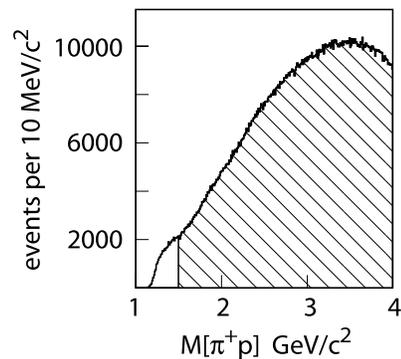
FIG. 5: Distribution in the  $\pi^+p$  effective mass for events in the charged mode satisfying the initial cuts. The shaded distribution shows the events accepted by the  $m_{\pi^+p} > 1.5 \text{ GeV}/c^2$  requirement.
