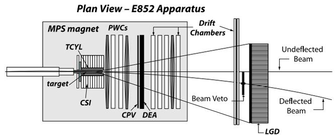
FIG. 1: E852 apparatus and the MPS at BNL.
