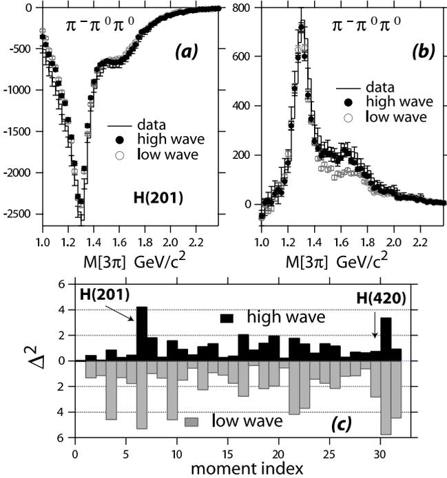
FIG. 16: Comparison of the (a)  $H(201)$  and (b)  $H(420)$  moments as computed directly from data and from PWA fits for the low and high wave sets for the  $\pi^-\pi^0\pi^0$  channel. In (c) the  $\Delta^2$  (differences squared divided by errors squared summed over all mass bins and divided by the number of mass bins) is shown for various moments.
