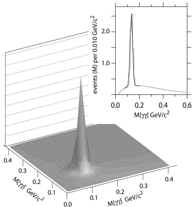
FIG. 2: Scatterplot of one di-photon mass against the other di-photon mass (three such pairings per event) for events satisfying the  $\pi^-\pi^0\pi^0p$  final state trigger and with four reconstructed photons in the LGD. The inset shows the di-photon mass spectrum with a fit to a Gaussian plus a polynomial. The  $\pi^0$  mass resolution is 10.4 MeV/c<sup>2</sup>.
