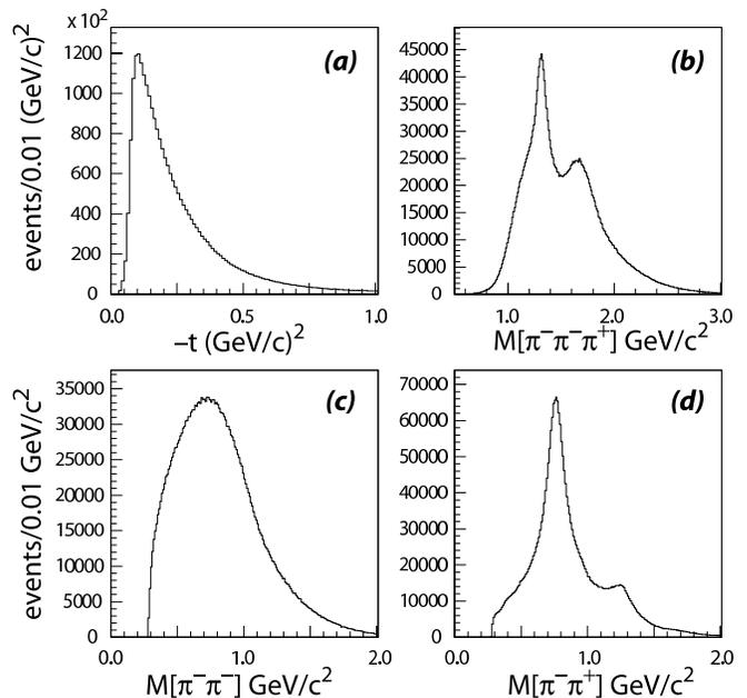
FIG. 7: (a) Uncorrected distribution in the square of the four-momentum transfer,  $t$ , from the incoming  $\pi^-$  to the outgoing  $(3\pi)^-$ ; (b)  $(3\pi)^-$  effective mass distribution; (c)  $\pi^-\pi^-$  effective mass distribution; and (d)  $\pi^-\pi^+$  effective mass distribution for the charged mode.
