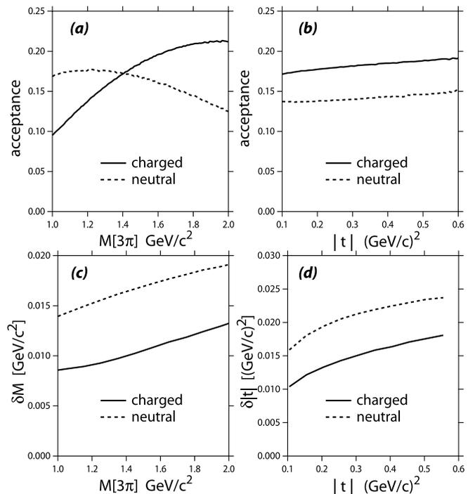
FIG. 10: (a)  $3\pi$  mass acceptance as a function of  $3\pi$  mass; (b)  $t$  acceptance as a function of  $t$ ; (c)  $\delta m$  – mass resolution as a function of  $3\pi$  mass; and (d)  $\delta t$  –  $t$  resolution as a function of  $t$  mass – all for both neutral and charged modes.
