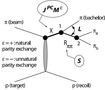
FIG. 12: Partial wave analysis of the  $3\pi$  system in the isobar model. The state  $X$  is characterized by spin ( $J$ ), parity ( $P$ ) and charge conjugation ( $C$ ). It decays at point 1 into a di-pion resonance  $R_{\pi\pi}$  (the isobar) and a bachelor  $\pi$ . The di-pion has spin  $S$ . The angular momentum between the isobar and the bachelor  $\pi$  is  $L$ . At point 2 the di-pion resonance decays into  $\pi_a$  and  $\pi_b$ . More details are given in the text.
