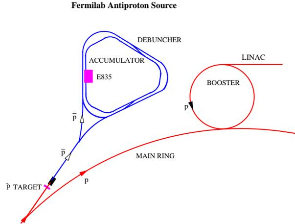
Figure 3.2: Schematic of the Fermilab Antiproton Source and its position relative to the FNAL Main Ring. The location of the E835 experiment in the Antiproton Accumulator is also shown.
