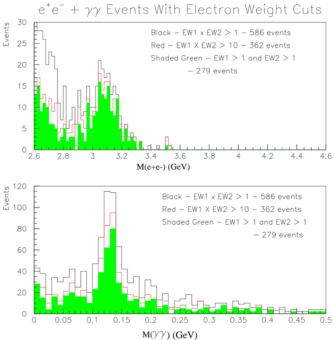
Figure 4.3: Effect of electron weight cuts on the  $M(e^+e^-)$  distribution for  $e^+e^- + \gamma\gamma$  events. Top figure shows the  $e^+e^-$  invariant mass for three choices of electron weight cuts. Bottom figure shows the corresponding  $\gamma\gamma$  invariant mass distributions.
