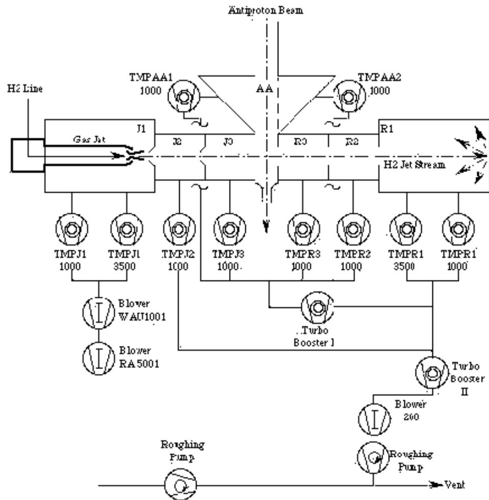
Figure 3.8: Layout of the hydrogen jet target and pumping system.
