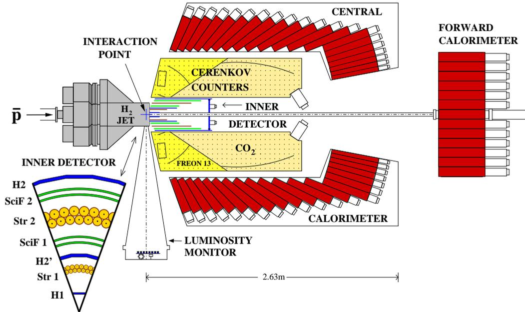
Figure 3.9: Side view of the E835 detector system.
