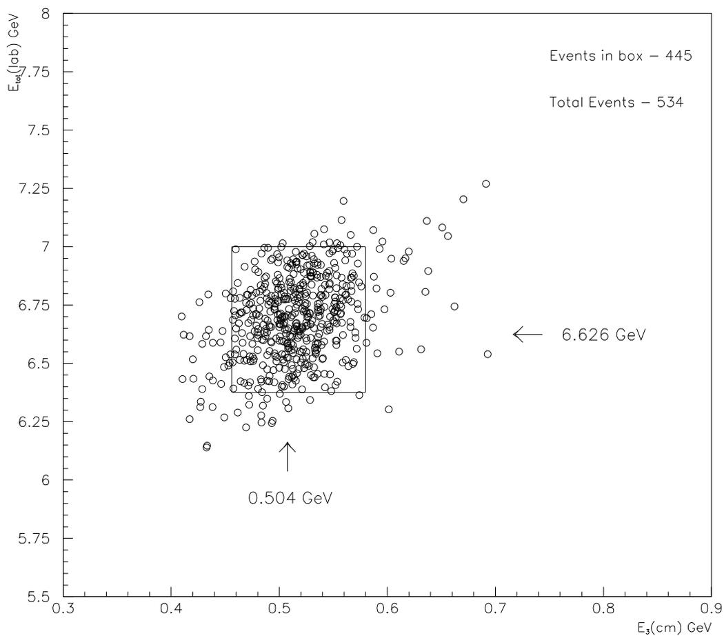
Figure 5.4: The  $E_{tot}(\text{lab})$  vs.  $E_{cm}(\gamma_3)$  distribution for all  $3\gamma$  events in the GEANT Monte Carlo with  $2.78 \text{ GeV} < M(\gamma_1\gamma_2) < 3.18 \text{ GeV}$ , and  $M(\gamma_1\gamma_3), M(\gamma_2\gamma_3) > 1.1 \text{ GeV}$  and  $|\cos(\theta^*)(\gamma_1, \gamma_2)| < 0.4$ . The box outlines the region in which  $6.376 \text{ GeV} < E_{tot} < 7.000 \text{ GeV}$  and  $0.454 \text{ GeV} < E(\gamma_3) < 0.580 \text{ GeV}$ .
