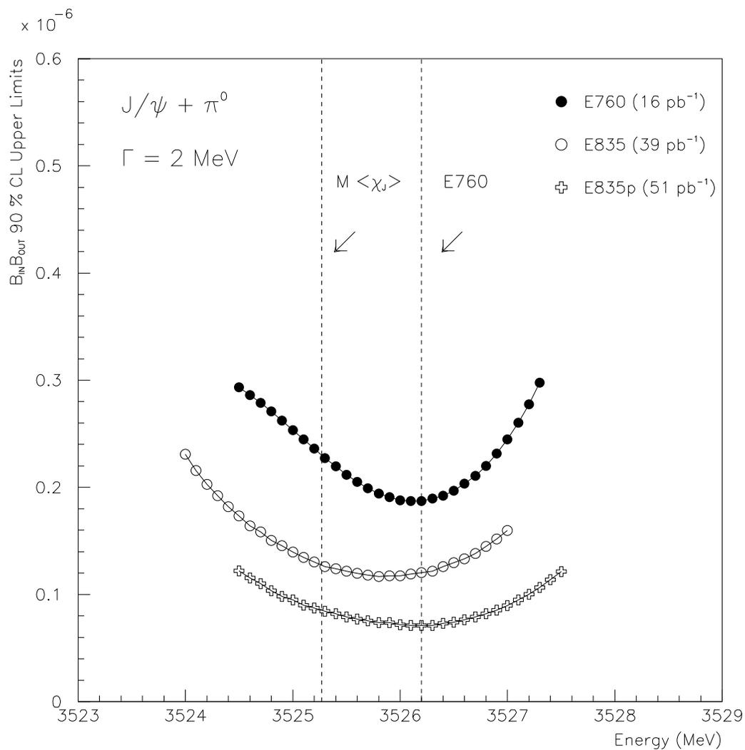
Figure 4.26: 90% CL upper limits for  $B_{in}B_{out}(p\bar{p} \rightarrow ^1P_1 \rightarrow J/\psi + \pi^0, J/\psi \rightarrow e^+e^-)$  for  $\Gamma(^1P_1) = 2$  MeV. The three curves shown show the results from the data from E760, E835, and E835p. The first vertical dashed line represents the center of gravity of the  $\chi$  states, and the second line shows the  $^1P_1$  mass value claimed by E760.
