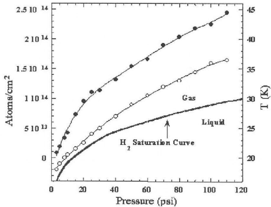
Figure 3.7: The  $P - T$  phase diagram for  $H_2$ . The operating points utilized by E835 are shown by open circles and the jet density corresponding to those operating points are shown by filled circles [93].
