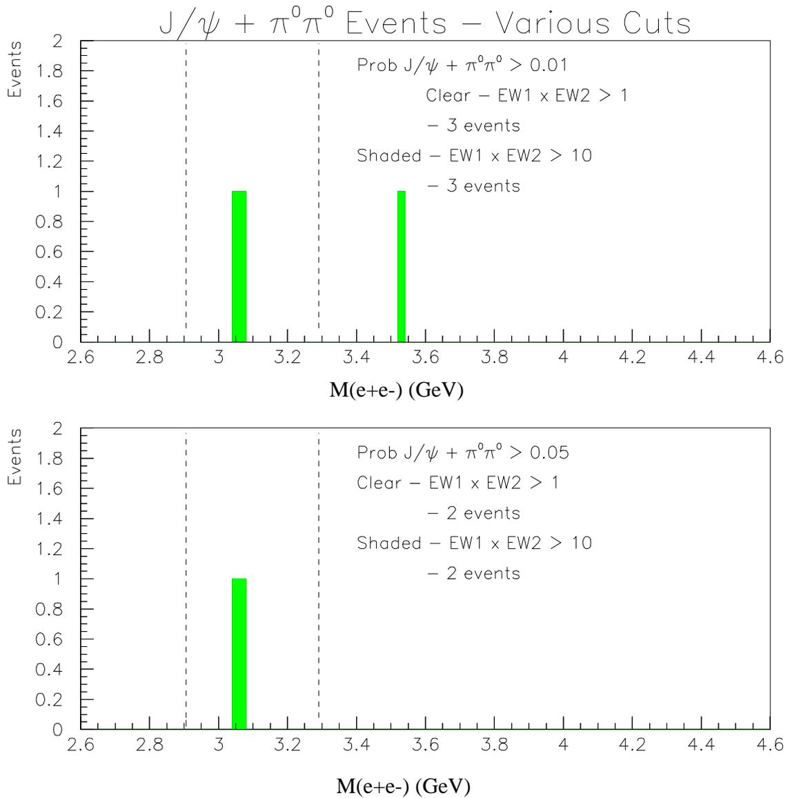
Figure 4.14: Effect of various electron weight and probability cuts on the  $M(e^+e^-)$  distribution for  $J/\psi + \pi^0\pi^0$  events. The top plot shows the  $M(e^+e^-)$  spectrum for  $P(J/\psi + \pi^0\pi^0) > 0.01$  and the bottom plot for  $P(J/\psi + \pi^0\pi^0) > 0.05$ . As in the previous channels, a final mass cut (dotted line) is made to remove events outside the region  $2.9 < M(e^+e^-) < 3.3$  GeV.
