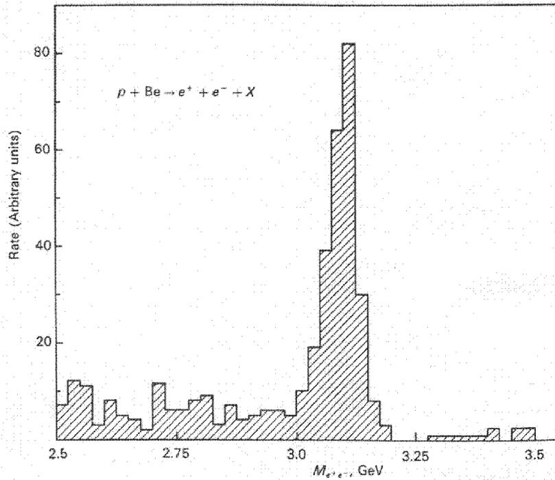
Figure 1.2: Results of Aubert *et al.* (1974) indicating the narrow resonance  $J/\psi$  in the invariant mass distribution of  $e^+e^-$  pairs produced in inclusive reactions of protons with a beryllium target. The experiment was carried out with the 28-GeV AGS at the Brookhaven National Laboratory. [10] [16]
