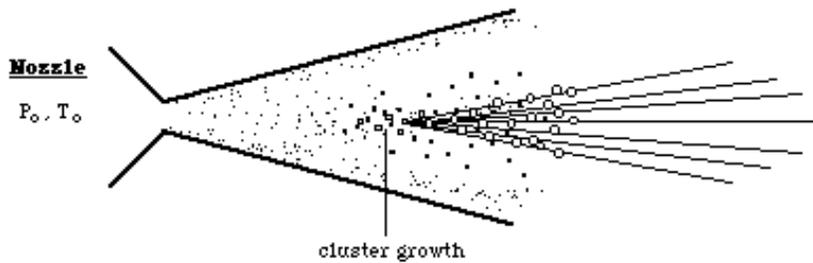
Figure 3.6: Detail of the gas jet nozzle and the formation of hydrogen clusters.
