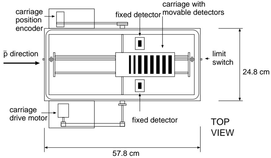
Figure 3.17: Schematic of the E835 luminosity monitor.
