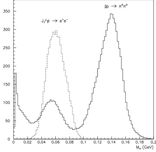
Figure 3.14: Distribution of the cluster mass for electrons and positrons using data from  $J/\psi$  decays (dashed), and from photons from a  $\pi^0\pi^0$  sample (solid). The large peak at  $M_{cl} > 100$  MeV is due to coalesced photons from the symmetric decay of the  $\pi^0$ .
