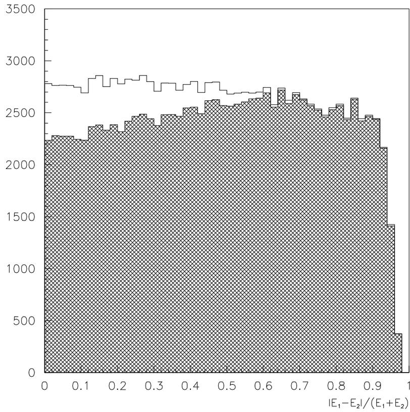
Figure 3.15: Distribution of the  $\pi^0$  asymmetry (data), defined as  $(E_1 - E_2)/(E_1 + E_2)$ , where  $E_1$  and  $E_2$  are the energies of the two photons. The distribution is plotted without the split clusters (shaded) and including the split clusters (open). The distributions are expected to be uniform.
