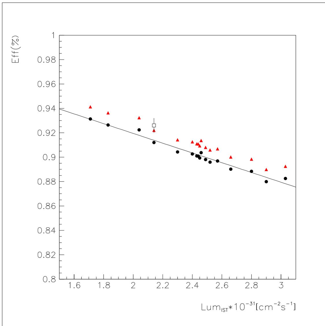
Figure 3.25: The probability that an  $e^+e^-$  event survives the pileup contamination versus the instantaneous luminosity, on a run by run basis [119]. The probability was calculated using random gate events collected at the  $\chi_0$  energy region. The black circles represent the efficiencies calculated using GEANT, and the red triangles represent the same efficiencies scaled to account for the difference between GEANT event and data events.
