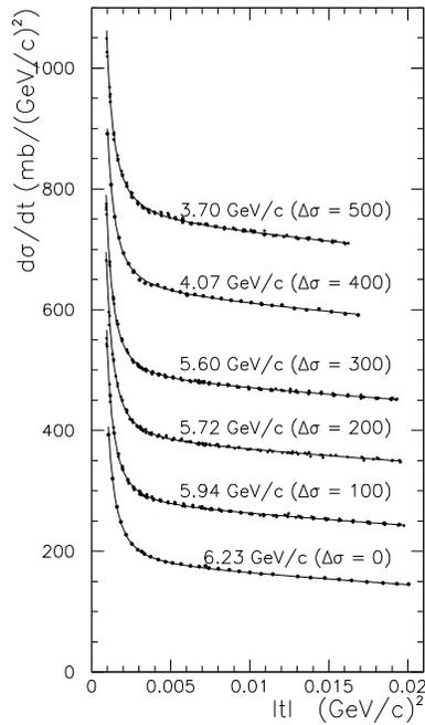
Figure 3.19: Measured  $p\bar{p}$  differential cross section,  $d\sigma/dt$ , versus squared momentum transfer,  $|t|$ , at six values of the  $\bar{p}$ -beam momentum (shifted vertically by an amount  $\Delta\sigma$  to distinguish them on the plot). Fits to the data are shown.
