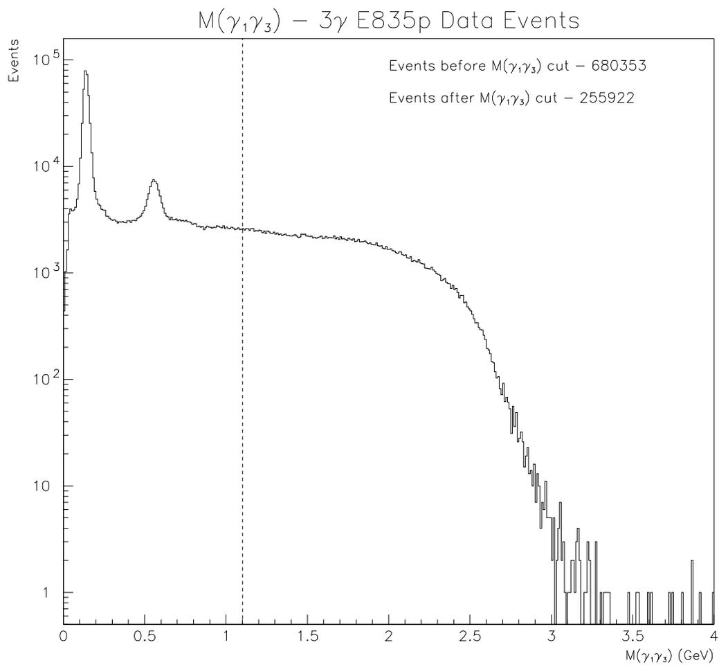
Figure 5.7: The  $\gamma_1\gamma_3$  invariant mass distribution for 3  $\gamma$  events in the E835p  $^1P_1$  data. The  $\pi^0$  and  $\eta$  peaks are clearly visible. Mass cuts are made to remove events with invariant mass  $M(\gamma_1\gamma_3) < 1.1$  GeV.
