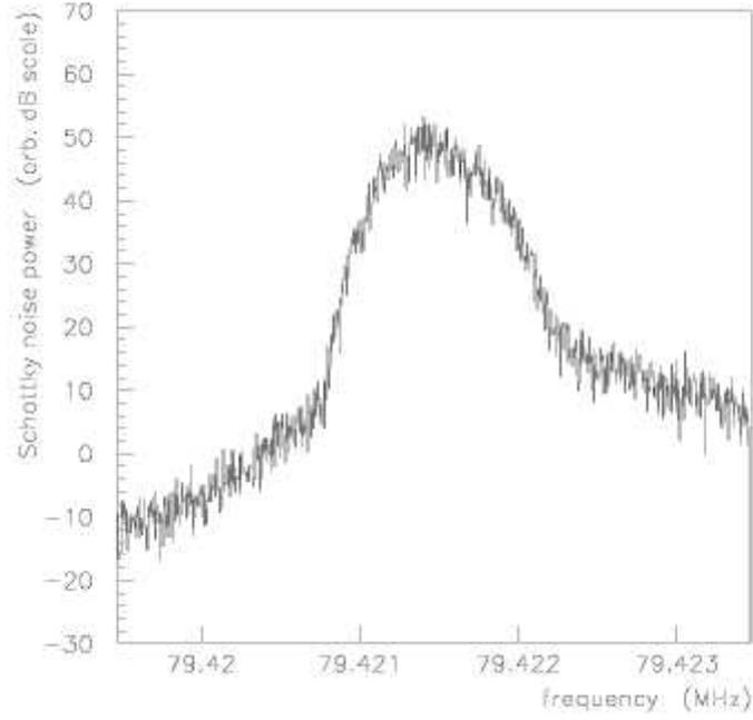
Figure 3.4: Measured Schottky noise power spectrum of the 127<sup>th</sup> harmonic of the antiproton beam with momentum 6232 MeV/c (the  $\psi'$  resonance). The central frequency is 79.421474 MHz [93]. An uncertainty  $\delta f$  of  $\sim 10$  Hz in the 127<sup>th</sup> harmonic corresponds to a  $\delta f$  of  $\sim 0.1$  Hz in the fundamental.
