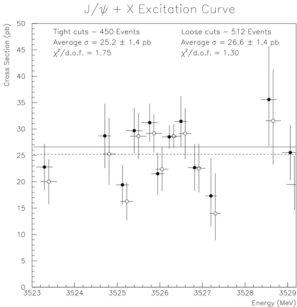
Figure 4.15: Efficiency corrected excitation curve for the  $J/\psi + X$  channel with **loose** electron weight cuts ( $EW1 \times EW2 > 10$ ) (closed circles) and **tight** electron weight cuts ( $EW1 > 1, EW2 > 1$ ) (open circles - slightly displaced). The cross sections are consistent despite different cuts. Stacks with energies less than 0.15 MeV apart have been combined.
