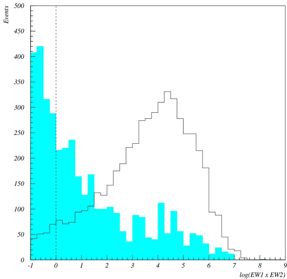
Figure 3.27: Comparison of electron weights of  $e^+e^-$  events and non-electron background events for all data taken in the  $\chi_1$  region. The dashed line represents the electron weight cut at  $EW1 \times EW2 > 1$ , which was used in the analysis of most of the decay channels in this thesis.
