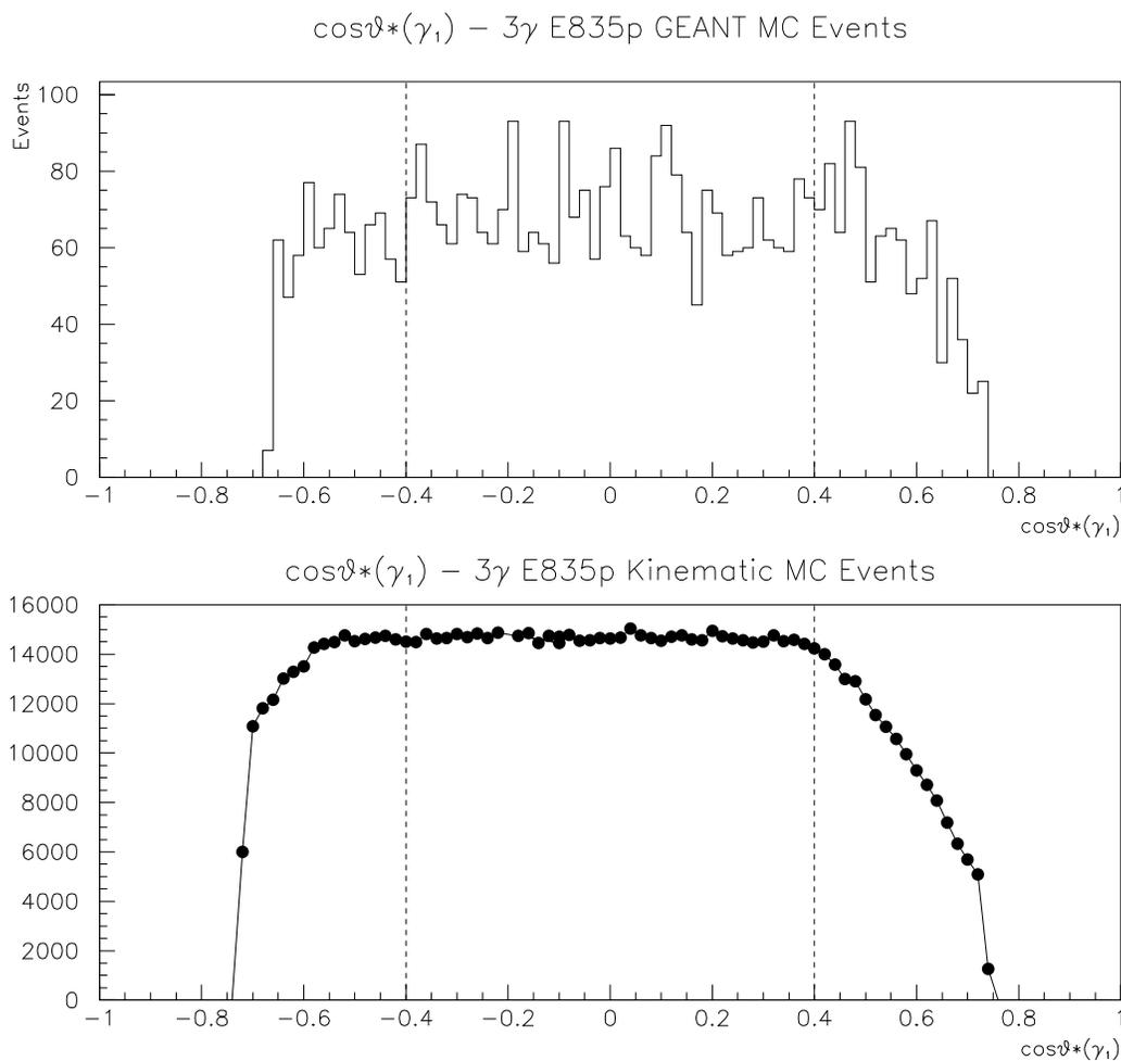
Figure 5.3: Top: The  $\cos(\theta^*)(\gamma_{1,2})$  distribution for all 3  $\gamma$  events in the GEANT Monte Carlo simulation of the reaction  $p\bar{p} \rightarrow {}^1P_1 \rightarrow \eta_c \gamma \rightarrow (\gamma_1 \gamma_2) \gamma$ . The vertical dashed lines show the cuts made to remove events with  $|\cos(\theta^*)(\gamma_1)| > 0.4$ . Bottom: The same plot made with a strictly kinematic Monte Carlo with 100 times the number of generated events.
