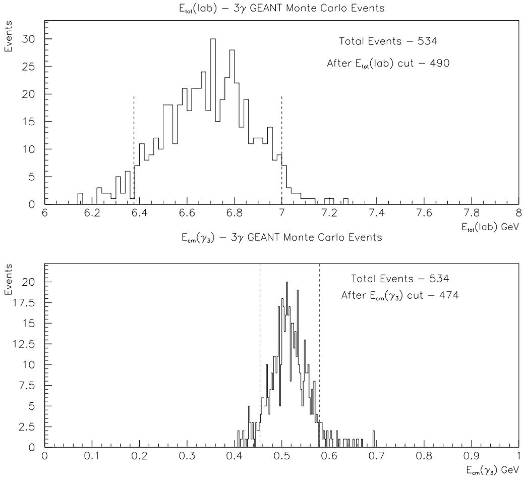
Figure 5.5: Top: The  $E_{tot}(\text{lab})$  distribution for all 3  $\gamma$  events in the GEANT Monte Carlo with  $2.78 \text{ GeV} < M(\gamma_1\gamma_2) < 3.18 \text{ GeV}$ , and  $M(\gamma_1\gamma_3), M(\gamma_2\gamma_3) > 1.1 \text{ GeV}$  and  $|\cos(\theta^*)(\gamma_1, \gamma_2)| < 0.4$ . Bottom: The  $E_{cm}(\gamma_3)$  distribution for the same GEANT Monte Carlo events.
