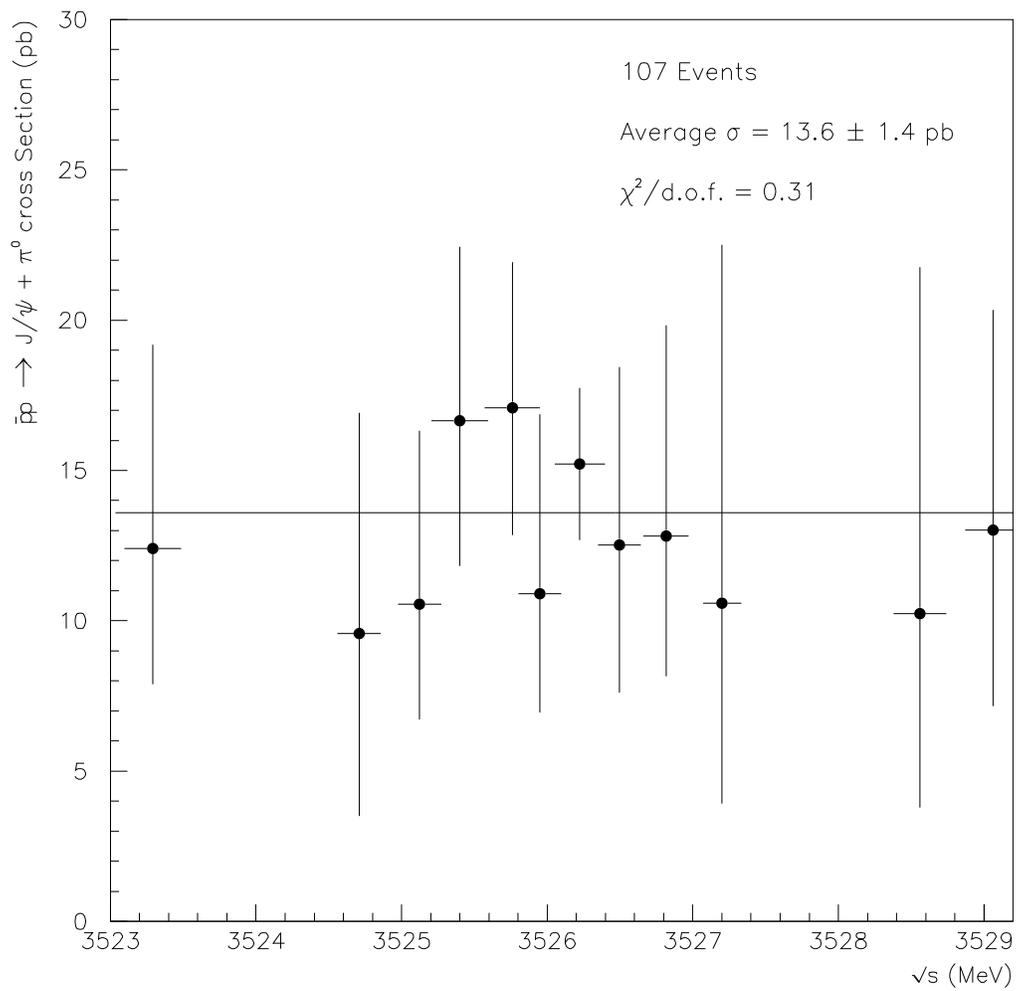
Figure 4.16: Efficiency corrected excitation curve for the  $J/\psi + \pi^0$  channel from the E835p data. Stacks with energies less than 0.15 MeV apart have been combined.
