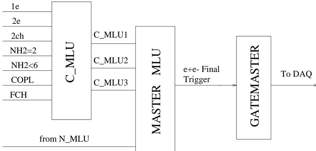
Figure 3.24: Schematic of the E835 charged trigger.
