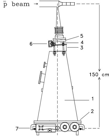
Figure 3.18: The E835 luminosity monitor as connected to the gas-jet target.
