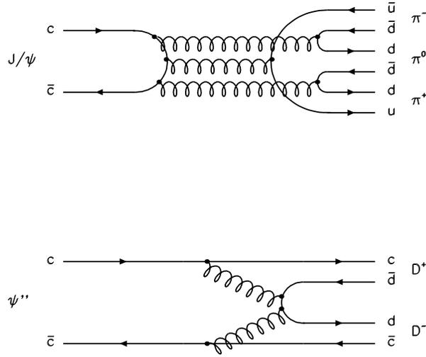
Figure 1.4: Examples of disconnected and connected diagrams. Top (a): the disconnected diagram of the decay  $J/\psi \rightarrow \pi^-\pi^0\pi^+$ . Bottom (b): the connected diagram of the decay  $\psi''(3770) \rightarrow D^+D^-$ .
