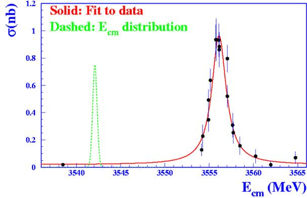
Figure 3.1: A scan of the  $\chi_{c2}$  resonance of charmonium using the E835 detector. The half width of the  $\chi_{c2}$  resonance is  $\sim 1.8$  MeV. The center of mass energy distribution of the beam, with typical half width of  $\sim 500$  keV, is shown by the dotted curve.
