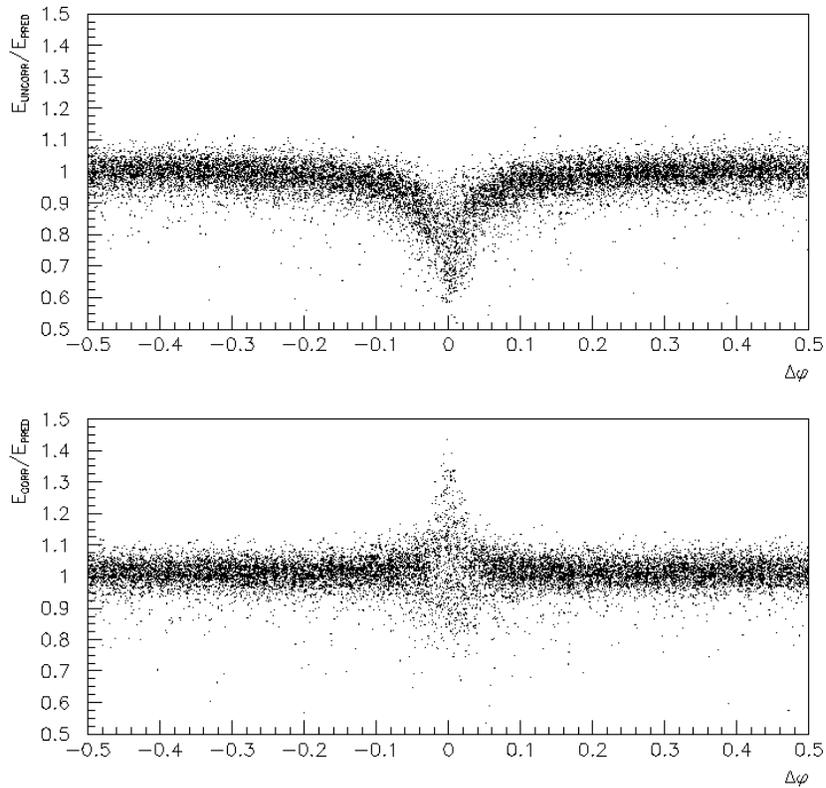
Figure 3.13: Ratio between the measured energy of the cluster and the energy predicted by the 2 body kinematics in  $J/\psi \rightarrow e^+e^-$  events, before (top) and after (bottom) energy correction, as a function of the distance from a CCAL crack.
