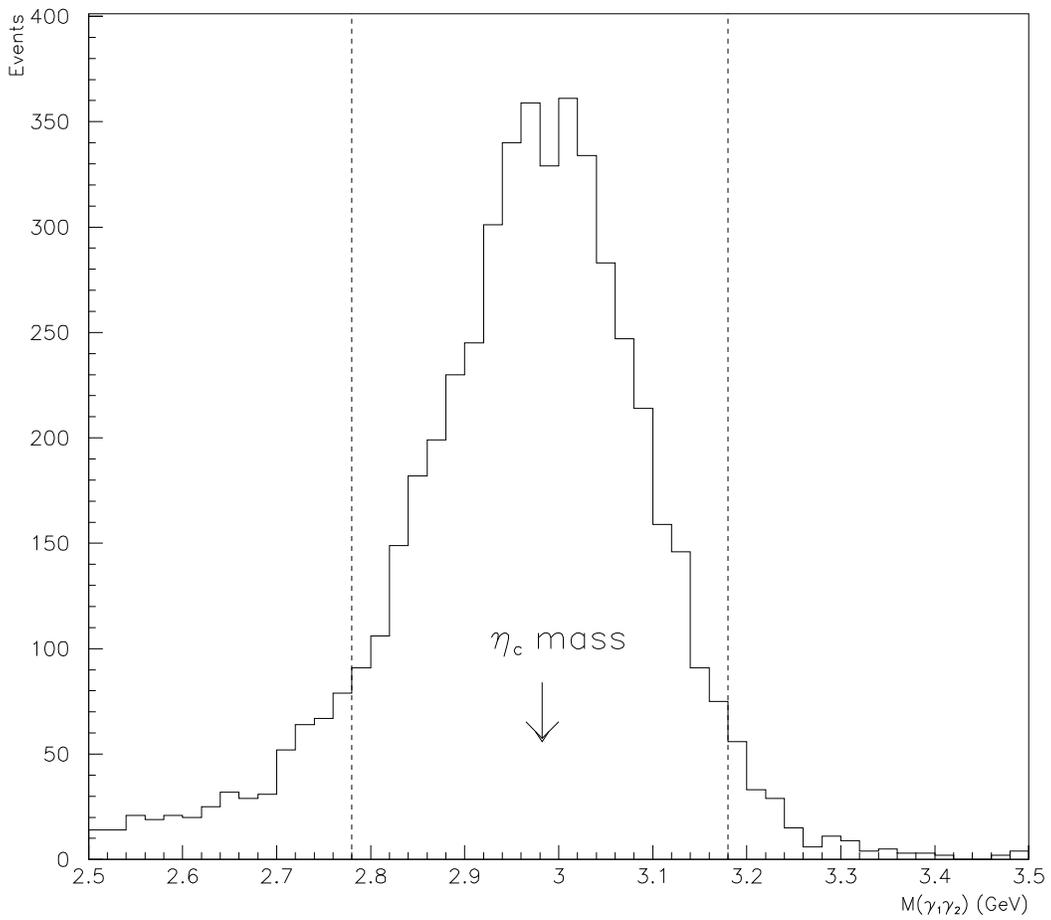
Figure 5.1: The  $\gamma_1\gamma_2$  invariant mass distribution for all 3  $\gamma$  events in the GEANT monte carlo simulation of the  $^1P_1 \rightarrow \eta_c\gamma \rightarrow 3\gamma$  decay channel.  $\eta_c$  mass cuts are made for events with invariant mass  $M(\gamma_1\gamma_2) < 2.78$  and  $M(\gamma_1\gamma_2) > 3.18$  GeV.
