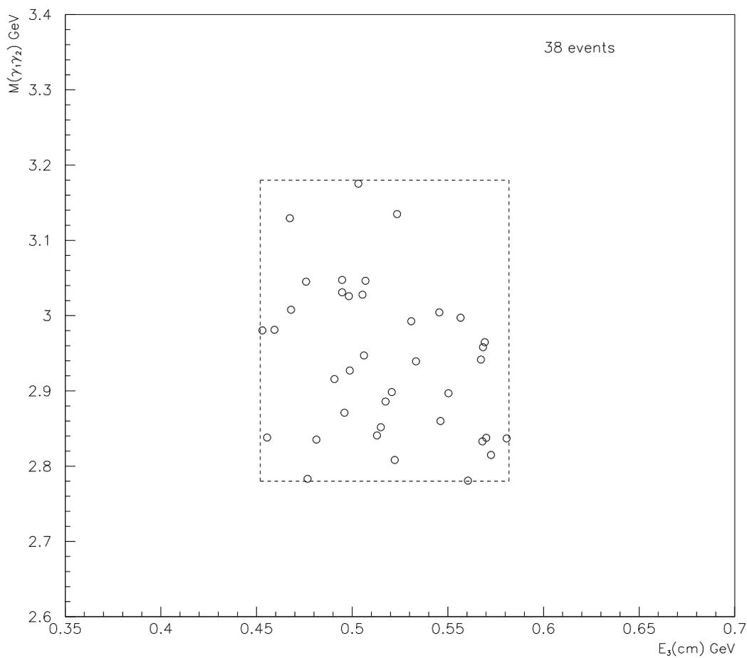
Figure 5.14: The  $M(\gamma_1\gamma_2)$  vs.  $E_{cm}(\gamma_3)$  distribution for all  $3\gamma$  events in the E835p  $^1P_1$  data in the final event selection, including cuts on  $E_{tot}(\text{lab})$  and  $E_{cm}(\gamma_3)$  as shown in Figs 4.38 and 4.39.
