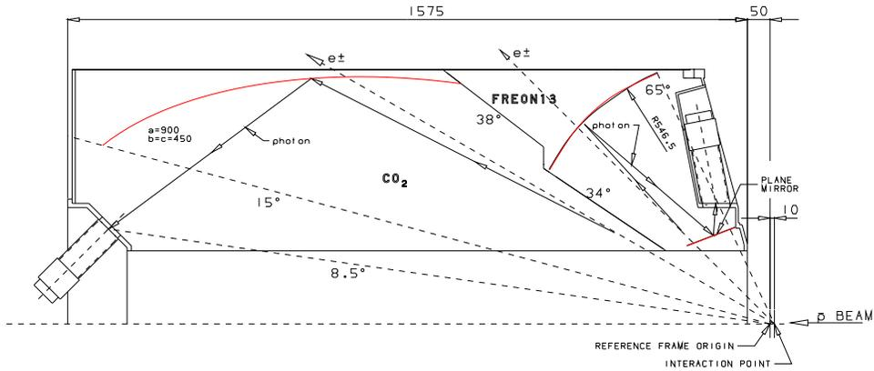
Figure 3.10: Schematics of the Čerenkov counter, showing one octant and its mirrors and angles. The septum at  $34^\circ/38^\circ$  divides each chamber into its forward and backward-angle cells. The spherical, plane and ellipsoidal mirrors are shown in red.
