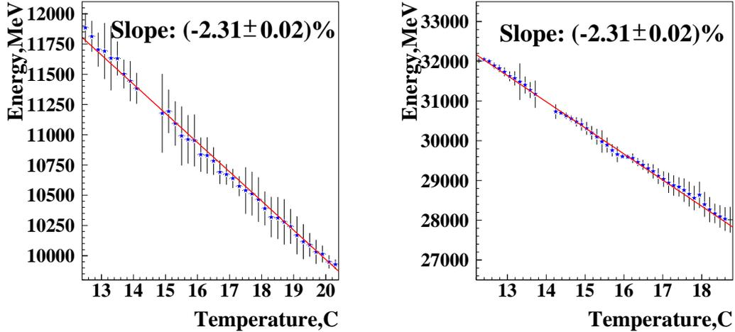
Fig. 10. Temperature dependence of light output for one of the crystals. Temperature in  $^{\circ}\text{C}$  is along the X-axis. Light output in terms of energy is along the Y-axis. Measurements were done with 10 GeV (left) and 27 GeV(right) electrons.
