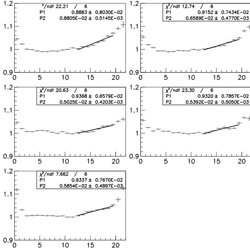
Fig. 3. Fit results for the energy loss distributions of 5 crystals as a function of the position along the crystal. PMT position is at the X=0 cm. LY on Y-axis were normalized to the LY at X=11 cm. Each plot corresponds to one crystal.
