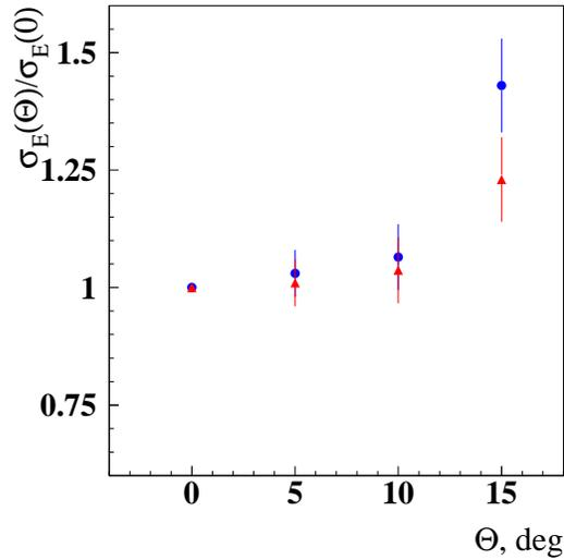
Fig. 9. Energy resolution dependence on the angle of electron incidence. Resolution along the Y-axis normalized to the resolution at  $0^\circ$ . Dots represent results from 27 GeV electron beam, triangles – 10 GeV electrons
