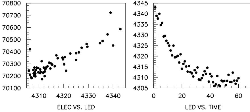
Fig. 5. (left) The correlation between the LED signal (on the X axis) and  $5 \times 5$  energy sum for electrons (on the Y-axis). (right) Dependence of the LED signal in ADC counts vs the time (on the X axis). Each point is an average over 90 seconds. Note, the highly suppressed zero on the scales. (All data are at 27 GeV.)
