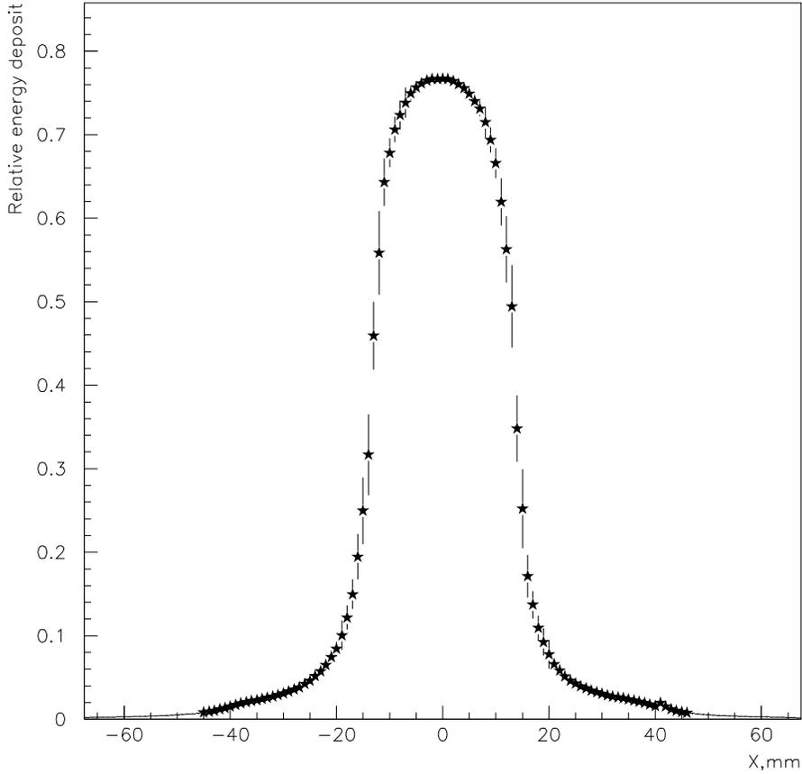
Fig. 11. Electromagnetic shower lateral profile for 45 GeV electrons.
