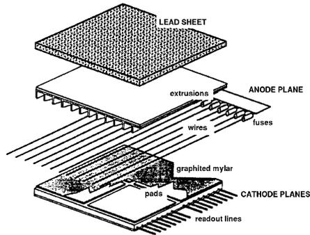
Figure 3.10: Portion of a separated ECAL layer.
