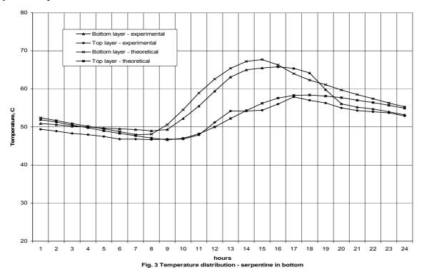
Results presented in fig.3 shows also the accuracy of other sub-problem in mathematical treatment. In time period between 22 and 7 o'clock there are not other thermal processes but heat loses to the ambient. Curves tilt in this period is the parameter, which is defined by thermal insulation of the accumulator. Presented results illustrate that heat loss coefficient  $U_{loss}$  for the
