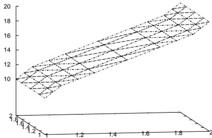
**Fig. 7.** Example finite element model the showing triangular elements. The height of each vertex corresponds to the solution value
