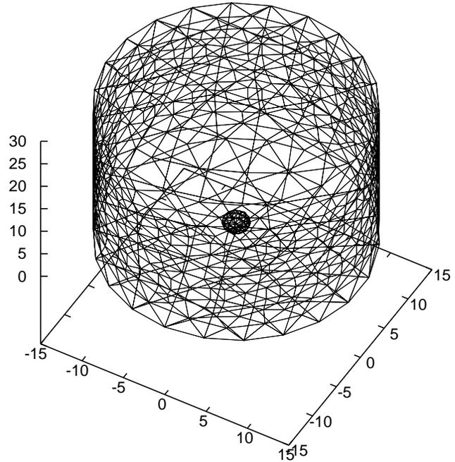
**Fig. 3.** Geometry of FEM model of phantom ball model from EIDORS project [9, 10]
