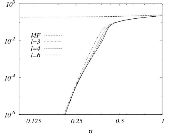
Fig. 2. The bit error rate as a function of the noise parameter  $\sigma$  at  $\alpha = 1.3$ . The bold continuous line is Tanaka's result for dense signatures under symbol MAP detection. MF refer to the same signature scheme under matched filter detection. The other (dashed) lines correspond to sparse signatures and BP detection.
