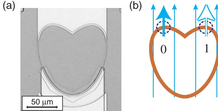
Fig. 5. (a) Photograph of a  $0.3 \mu\text{m}$  wide heart-shaped junction fabricated in Nb-AlO<sub>x</sub>-Nb technology. (b) Sketch of heart-shaped junction with magnetic field applied along the symmetry axis of the junction. Two energetically identical vortex states are indicated by arrows in positions 0 and 1.
