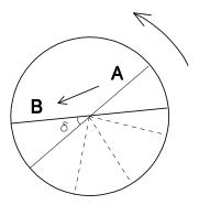
FIG. 1. The avalanche mixing scheme in the case of a half filled drum. When the free surface slope attains the marginal stability angle value, the granules of different fractions flow quickly from sector A to sector B, undergoing mixing. Then the free surface slope turns to be equal to the repose angle of the material under consideration. The angle  $\delta$  is the difference between the angle of marginal stability and the angle of repose. The mixing fractions are not shown.
