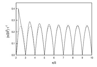
FIG. 2. Scaled inverse avalanche mixing time  $(\pi/2\delta^2)\tau^{-1}$  vs.  $\pi/\delta$ . The solid line is obtained from the "exact" solution of the characteristic polynomial (9). The dashed line represents expression (8) which is, formally speaking, obtained in the limit of small  $\delta \ll \pi$ .
