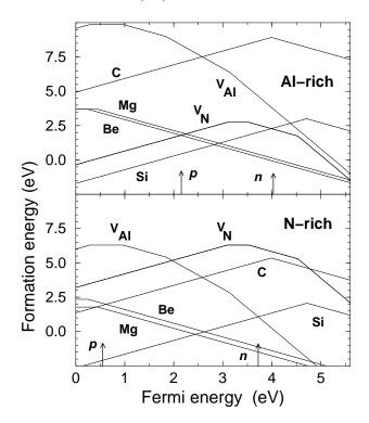
FIG. 1. Formation energy of impurities and native defects in AlN, for N-rich and Al-rich growth conditions. Arrows indicate the best Fermi levels achievable in typical conditions ( $T_q \sim 1200$  K).
