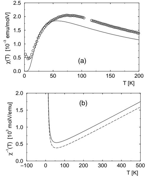
FIG. 4. (a)  $\chi(T)$  from model parameter set. Deviations from measured data<sup>10</sup> are discussed in text. (b)  $\chi^{-1}(T)$  with (solid line) and without (dashed) mean-field correction.
