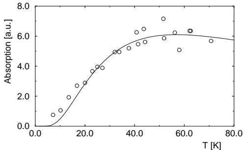
FIG. 5. ESR absorption from model parameter set, showing excellent consistency with observation.<sup>10</sup>
