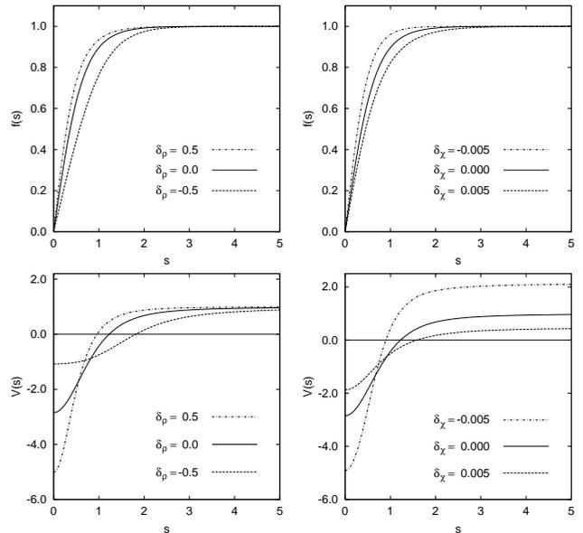
FIG. 1. A display of the vortex cores for various values of the anisotropy parameters. Graphs of the modulus  $f(s)$  of the superconducting order parameter as well as of the effective potential  $V(s)$ . The parameters are  $\kappa = 84$  and  $\gamma = 1.014$ . When  $\delta_\rho$  is varied,  $\delta_\chi = 0$  and vice versa.
