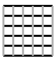
Fig 1. A schematic of the array discussed in the text; the solid (shaded) lines are the horizontal (vertical) superconducting wires that are coupled by Josephson junctions to the vertical (horizontal) wires at each node.
