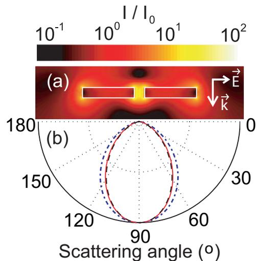
FIG. 3: (color online) (a) Near field intensity at the longitudinal resonance for an antenna with strongly coupled arms ( $\Delta = 20$  nm,  $L = 100$  nm). (b) Far-field scattering pattern of the antenna (solid line, red), together with the emission patterns of a point dipole (dash-dotted line, blue), and a half-wave antenna (dashed line, black).
