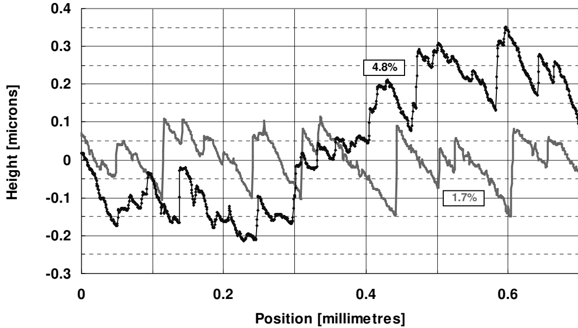
Figure 2. Surface profiles of a KCl single crystal deformed in compression along the [100] axis to compressive strains \epsilon = 1.7\% and \epsilon = 4.8\% .
