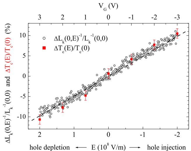
FIG. 3: Comparison of the field-induced relative changes of the critical temperature and of the inverse kinetic inductance at very low temperature ( $T = 0.6$  K,  $T/T_c \approx 0.07$ ) for an underdoped ( $x = 0.1$ ) 2-UC-thick LSCO film as a function of the applied electrostatic field. The dashed straight line is a fit according to Eq. (2).
