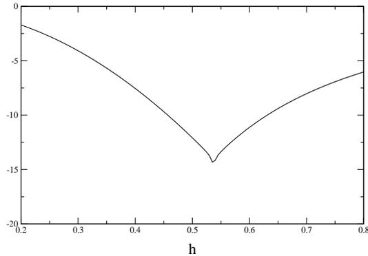
FIG. 2:  $\log_{10} |E_0 - E_0^{exact}|$  as a function of the spacing  $h$  using  $k_{max} = 10$  for the harmonic oscillator  $V(x) = x^2/2$ .
