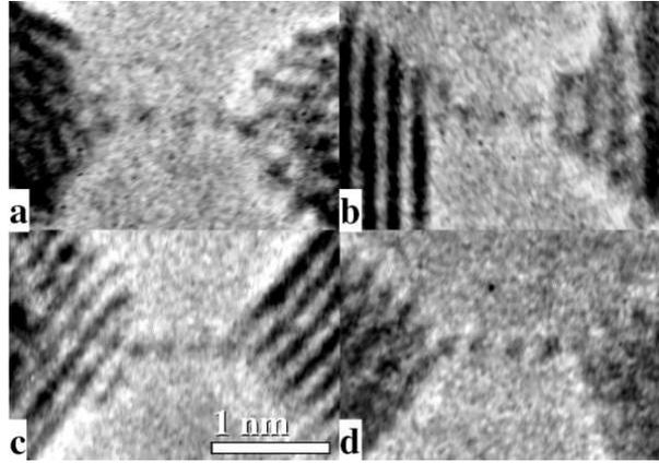
FIG. 2: a-d) Atomic resolved HRTEM snapshots of suspended atom chains generated from different alloy compositions  $\text{Au}_{1-x}\text{Ag}_x$ , for  $x=0.2$ ;  $0.4$ ;  $0.6$  and  $0.8$ , respectively. Atomic positions appear dark. See text for explanations.
