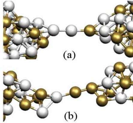
FIG. 5: Snapshots from the molecular dynamics simulations showing the formation of mixed LACs from alloys: (a)  $\text{Au}_{40}\text{Ag}_{60}$  and (b)  $\text{Au}_{60}\text{Ag}_{40}$ . Yellow (gray) indicate gold (silver) atoms.
