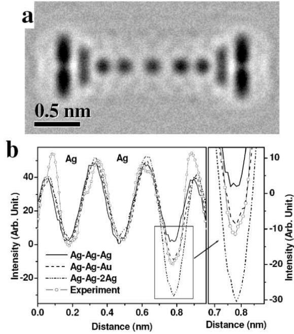
FIG. 3: a) HRTEM simulated image of a mixed atom chain formed by three suspended atoms hanging between to Ag tips, the LAC is formed two Ag atoms and a Au one at the right end. b) Comparison between experimental ( $\text{Au}_{20}\text{Ag}_{80}$ ) and simulated intensity profiles across a metal alloy LAC formed by three hanging atoms (see text for discussions). Atomic positions appear as intensity minima and are indicated by arrows in the profile.
