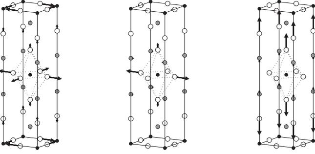
FIG. 5: Displacement patterns of the high-frequency oxygen bond-stretching modes of LaCuO. Left: planar breathing mode ( $O_B^X$ ), middle: half-breathing mode ( $\Delta_1/2$ ), right: apex-oxygen breathing mode ( $O_Z^Z$ ).
