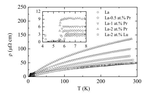
FIG. 3: Temperature dependence of the electrical resistivity of some of the samples studied. Inset: Detail around the superconducting transition.
