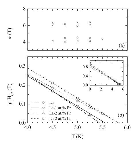
FIG. 5: Some examples of the temperature dependences of (a) the Ginzburg-Landau parameter and (b) the upper critical magnetic field. These quantities were obtained from  $M(H)_T$  measurements like the ones shown in Fig. 4. In the inset of Fig. 5(b) it is presented a linear extrapolation of  $\mu_0 H_{c2}(T)$  to T=0 K.
