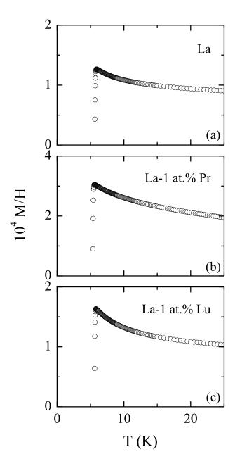
FIG. 2: Some examples of the temperature dependence of M/H measured under low magnetic fields (in these examples with  $\mu_0H=50$  mT) for three of the superconducting compounds studied in this work.
