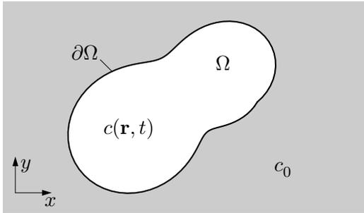
FIG. 1: A sketch of the cross section  $\Omega$  (white) with boundary  $\partial\Omega$  (black curve) in the  $xy$ -plane of a rod with translational invariance in the  $z$  direction. At time  $t = 0$ , where the concentration  $c(\mathbf{r}, t)$  inside  $\Omega$  is zero, diffusion is suddenly turned on from the outside, where the concentration is kept at the constant value  $c_0$  (gray).
