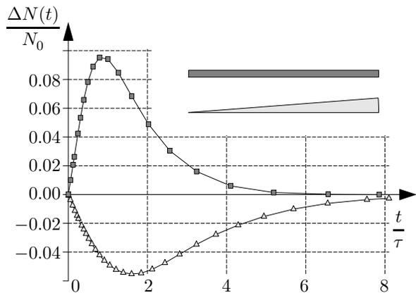
FIG. 4: Plots as in Fig. 3 but here for two extreme geometries: a sector of a circular disc with angle  $2 \arctan(1/30)$  and a rectangle with aspect ratio  $1/30$ , see insets. While these two shapes have nearly the same area and perimeter, the former fills slower than the circular cross section and the latter faster. The maximal deviations are  $-6\%$  and  $+10\%$ , respectively.
