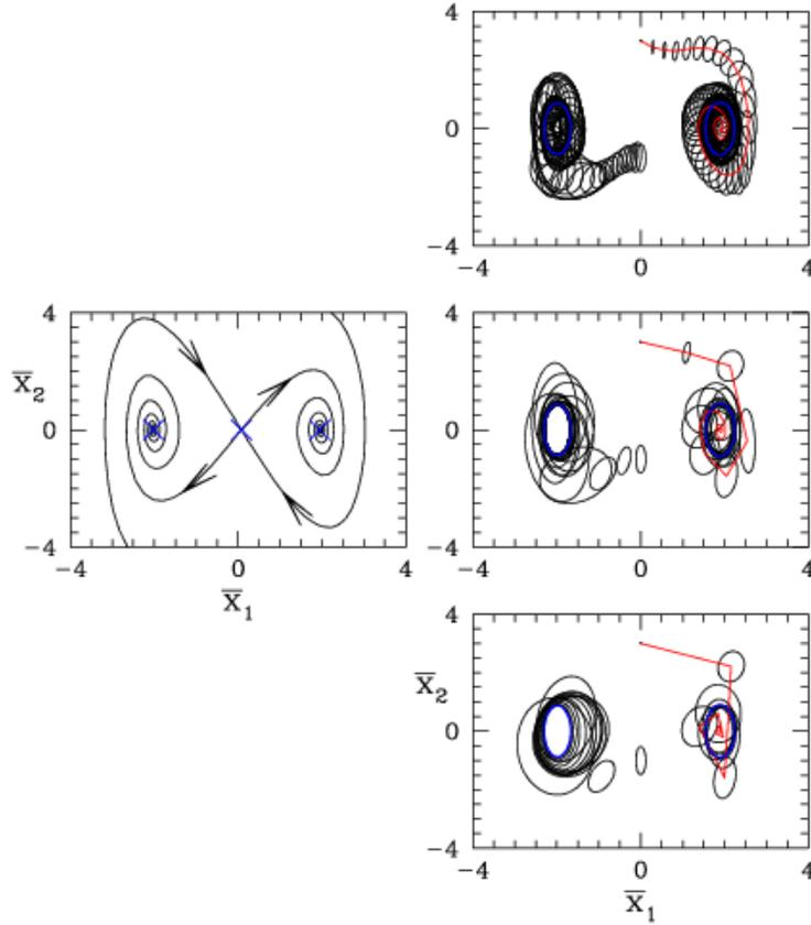
FIG. 4.19. Phase portraits showing the dynamics of moment maps for the heat bath model. First-order (left) and second-order (right) maps are shown. For the first-order map  $N = 8000$  particles is used. For the second-order map the following are used: (top)  $N = 256000$ ,  $\tau = 0.1$ ; (middle)  $N = 8000$ ,  $\tau = 0.4$ ; (bottom)  $N = 1000$ ,  $\tau = 0.8$ .
