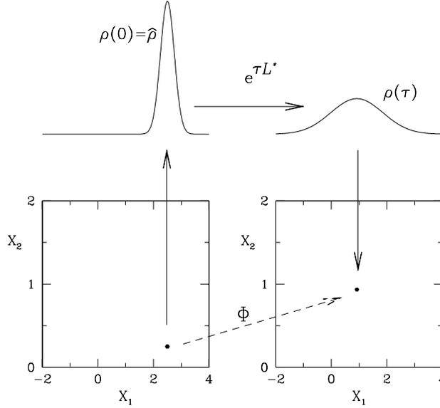
FIG. 3.1. Sketch illustrating the definition of the moment map. From a point  $(X_1, X_2)$  in moment space a density  $\hat{\rho}$  is uniquely determined. This initial density is evolved by the system dynamics (e.g. the Fokker-Planck equation). From the resulting density  $\rho(\tau)$ ,  $\tau$  time units later, a new point in moment space is determined. This point is defined to be the image of  $(X_1, X_2)$  under the moment map.
