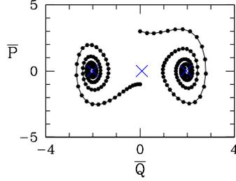
FIG. 1.4. Dynamics of a moment map for the first-order moments of the position  $Q$  and momentum  $P$  of the distinguished particle. The map has three fixed points; two stable foci and one unstable saddle shown as blue cross. Two trajectories are shown; one evolving to each of the stable fixed points. The right trajectory has initial condition  $(\bar{Q}, \bar{P}) = (0, 3)$ , corresponding to that in figure 1.3. There are  $N = 8000$  particles in the heat bath.
