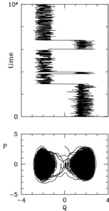
FIG. 1.2. Typical behavior for the dynamics of the distinguished particle in contact with a bath with  $N = 8000$  particles. Most of the time the distinguished particle is located in one of the two potential wells, but occasionally it makes a jump between wells.
