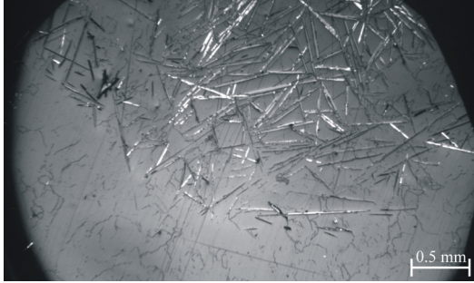
FIG.2. Etching pattern of a \text{ZrB}_{12} single crystal cross section in (100) plane from the same parts of ingot as in [19, 23]. The needle like long grains are \text{ZrB}_2 phase, while the small black lines correspond to etching pits from small angle boundaries.
