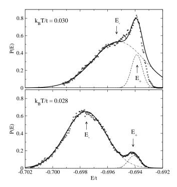
FIG. 4: Probability distribution of the energy at temperatures close to the critical temperature for U/t=0.5. The thick solid lines represent a superposition of two Gaussians that fit the simulation results, whereas the dashed and dasheddotted lines show the component Gaussians. The arrows indicate positions of the centers of the Gaussians representing low-temperature  $(E_{-})$ , and high-temperature  $(E_{+})$  phases, respectively.
